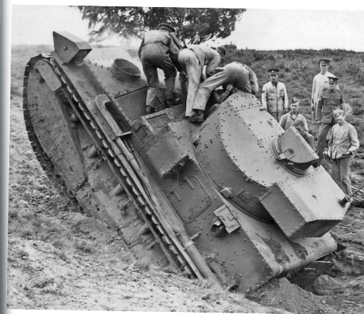
A rare top view of a Mark II** stuck in a hole showing the Bishop's mitre cupola and the wireless bulge, complete with aerial. Notice too the tinplate cowl over the nearside headlight. This was intended to mask the beam at night from the air.
