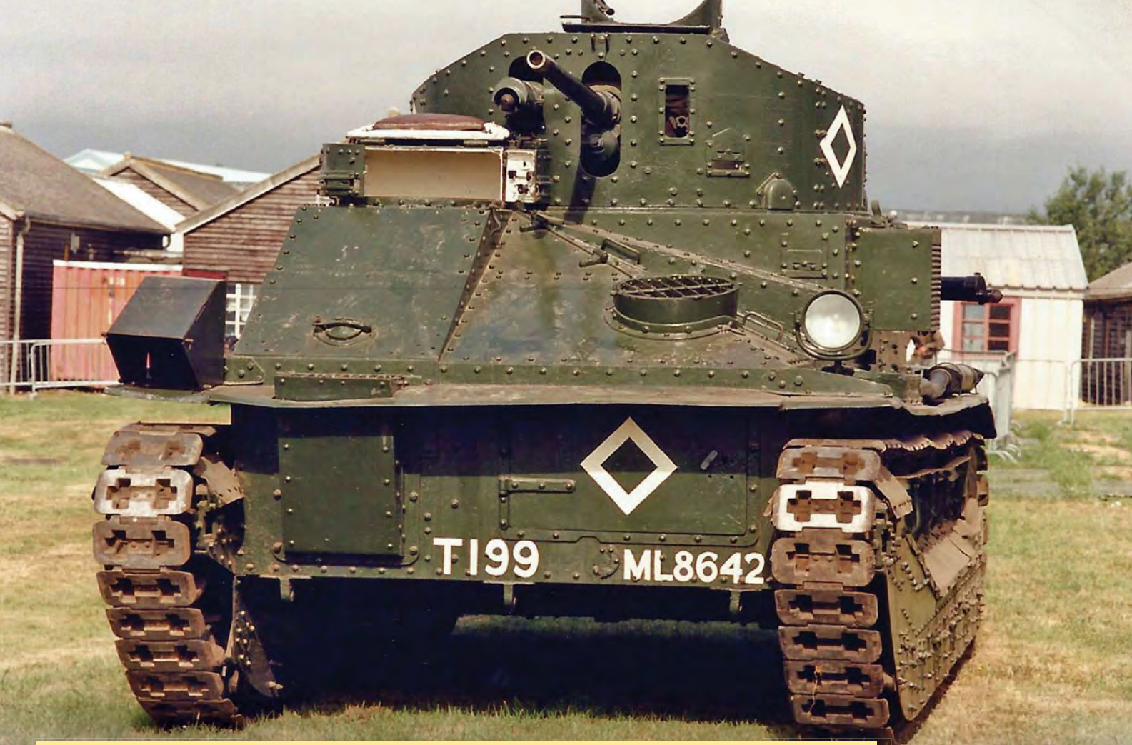
This Mark II* is the Tank Museum exhibit, displaying the Bishop's mitre cupola and the co-axial machine gun mounting.
