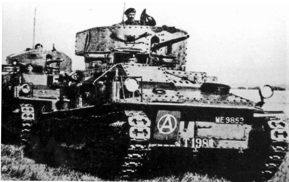
T198 started life as an ordinary Medium Mark II but was later modified into a command tank with a special turret. We know very little about it.
