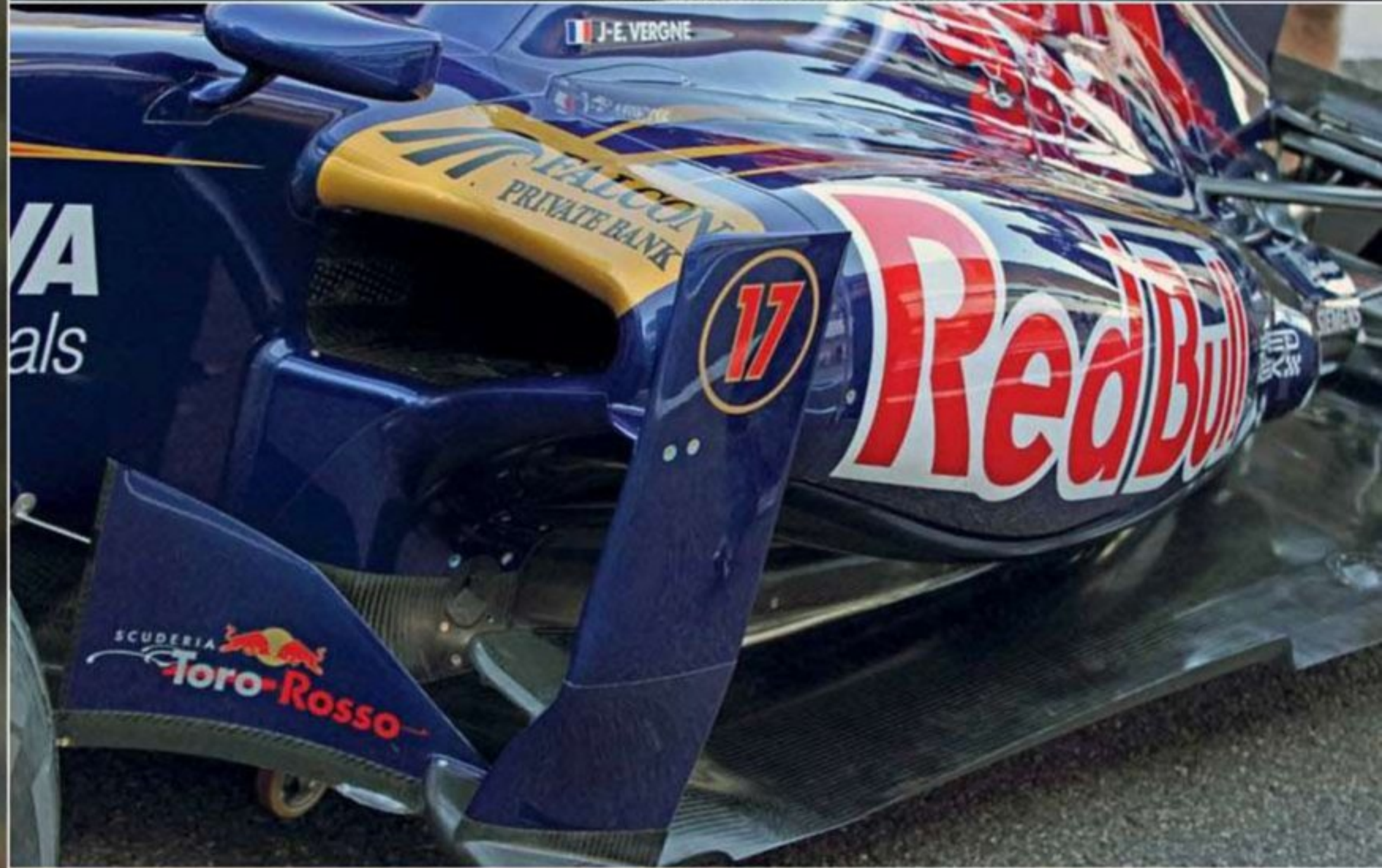
Top: The STR7 started the season with very basic exhaust exits as the team had struggled to simulate the plume in the wind tunnel. New facilities lead to a better understanding and the installation of a Coanda style exhaust. Above: The heavily undercut sidepods on the Toro Rosso are one of its defining features, this raises the centre of gravity of the cooling system but has a number of aerodynamic gains
