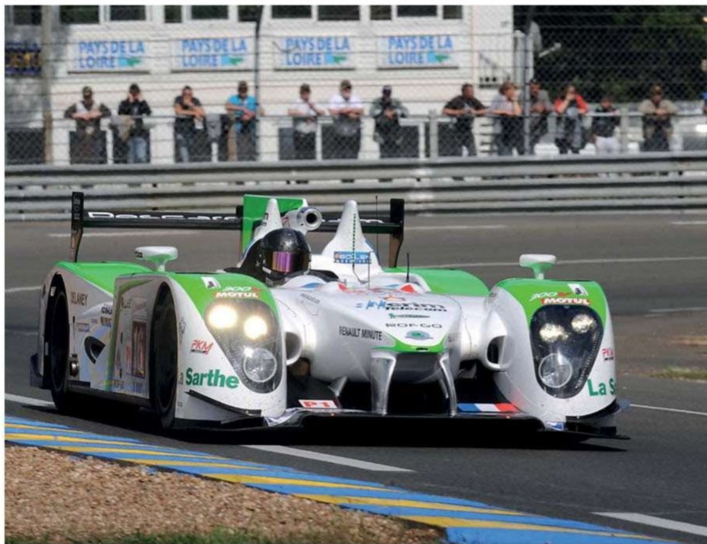
The Nick Perrin designed Pescarolo 03 featured the Aston Martin AMR-One chassis, and the Judd DB V8 engine
