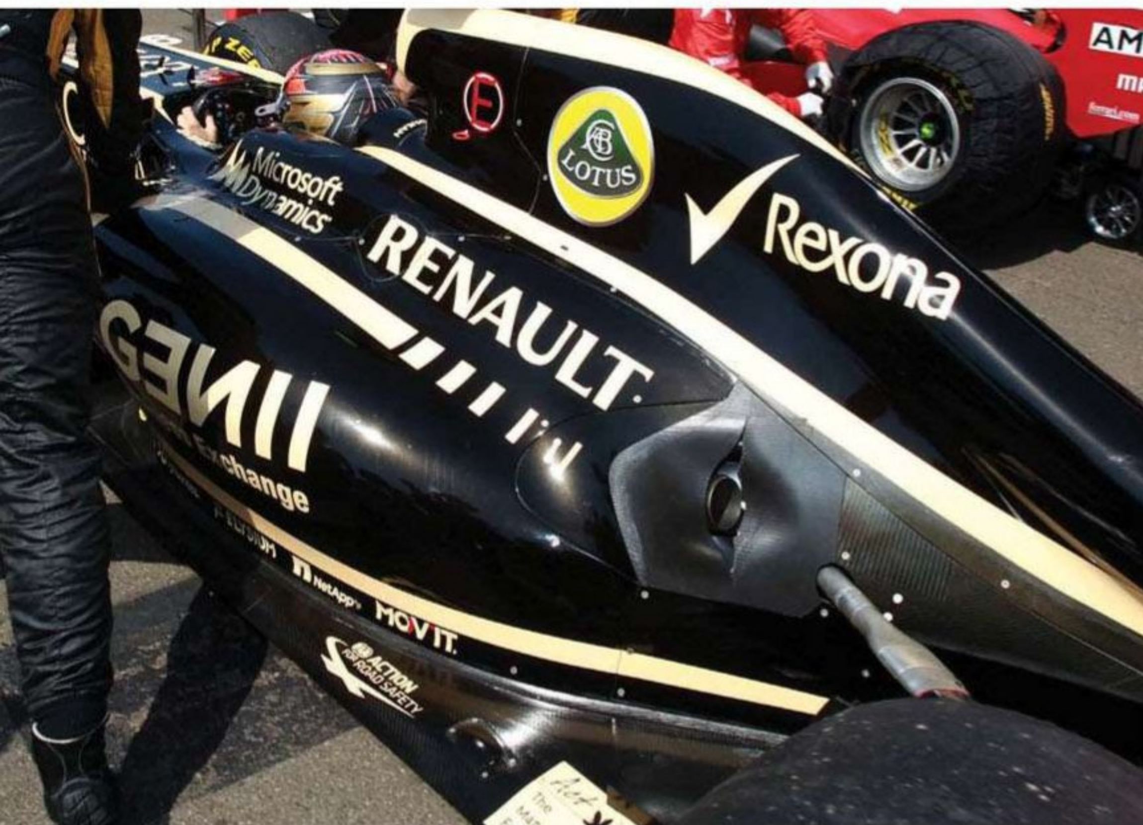
Lotus ran 'plain jane' exhausts on the E20 for most of the year, but finally fitted the more effective Coanda exhausts at the Korean Grand Prix in October
