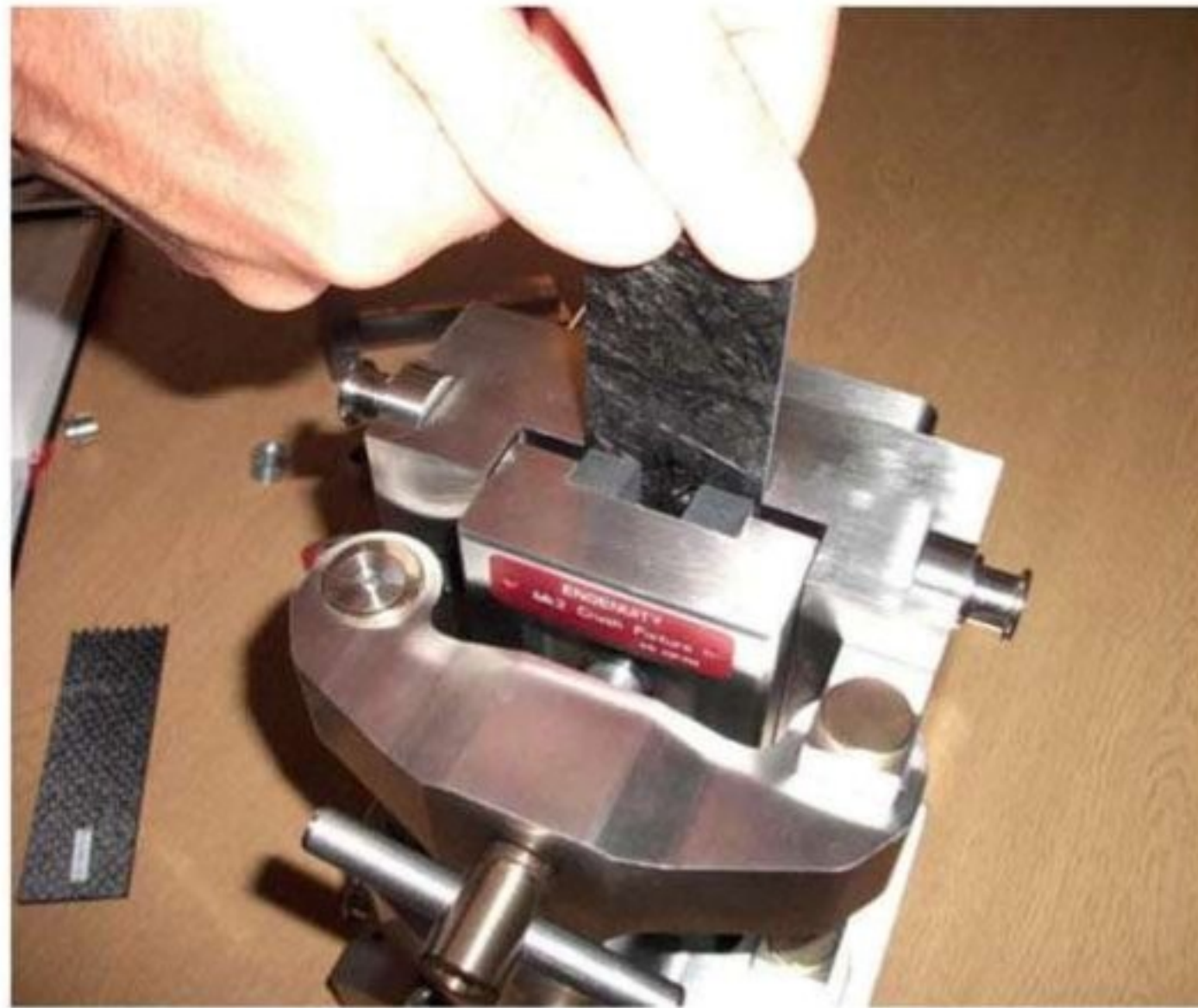
Carbon Fibre crush testing fixture at Engenuity gathering real-world performance data
