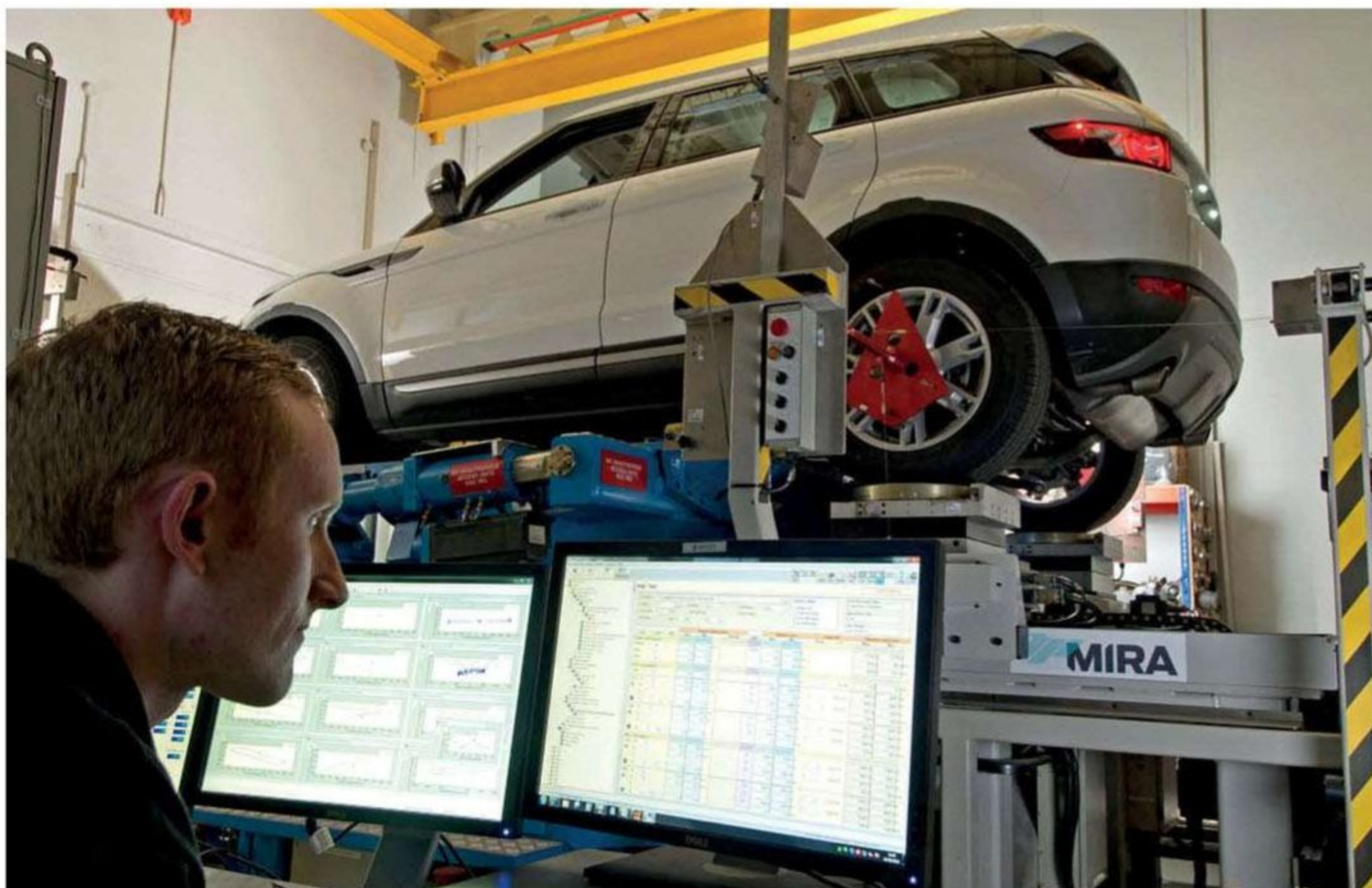
Discovering the vehicle's DNA on the MIRA Kinematics and Compliance (K&C) rig where suspension characteristics can be gathered and verified
