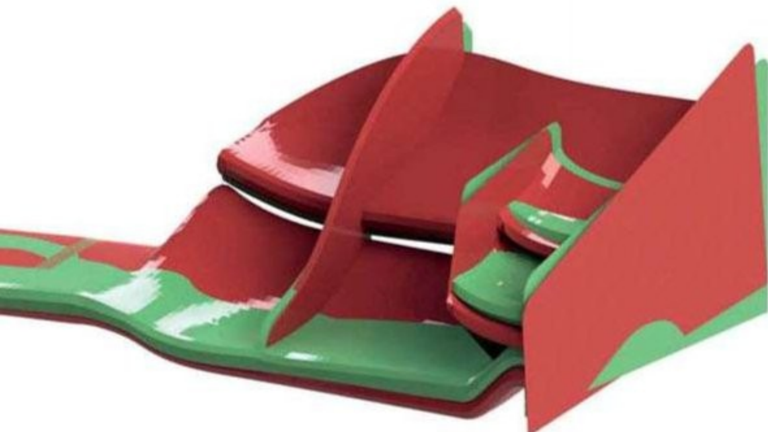
Figure 7: the red wing is the original, the green wing is the optimised one; note again how the green wing bends less but twists back more under aerodynamic load. Yet it met the prevailing FIA test load
