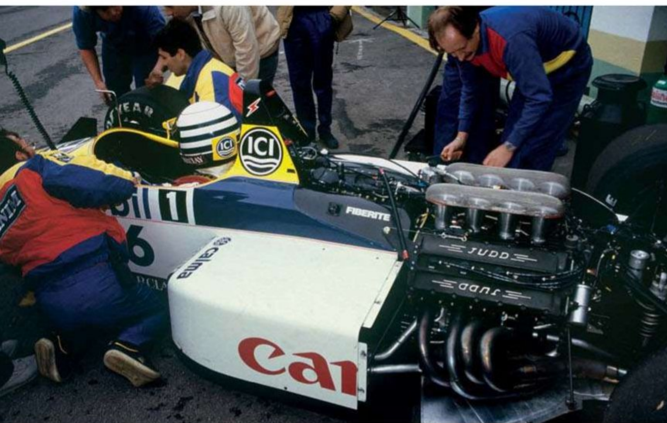
Judd spent a decade in Formula 1, supplying Williams with a 3.5 litre V8 in the FW12
