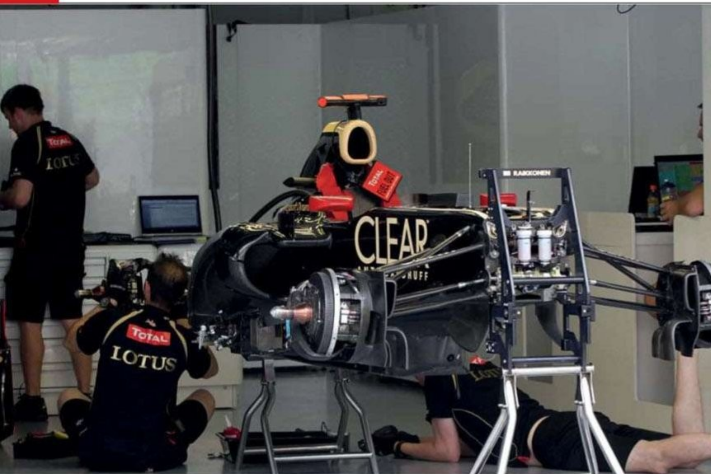
The E20 is a fairly conventional 2012 F1 design, with pullrod rear suspension and pushrod front suspension. Note the side impact structures sitting just forward of the sidepod duct
