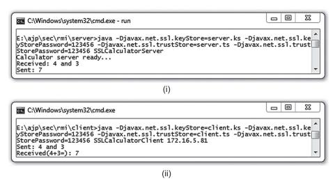
Figure 19.7: RMI over SSL using client authentication (i) Server (ii) Client
