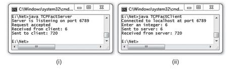
Figure 13.11: Communication using TCP socket (i) TCPFactServer (ii) TCPFactClient The execution timeline is also shown in Figure 13.12:
