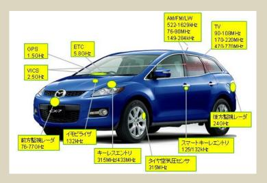
It is said that the "largest sources of electromagnetic waves" in automobiles are the power train (engine, motor, battery) and tires, but of course these are "sources of electromagnetic waves as by-products". All common devices and equipment
