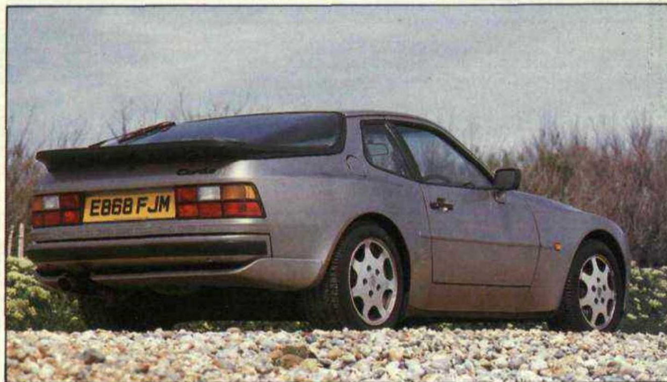
Rear under-lip helps to cool the aft-mounted transaxle.
