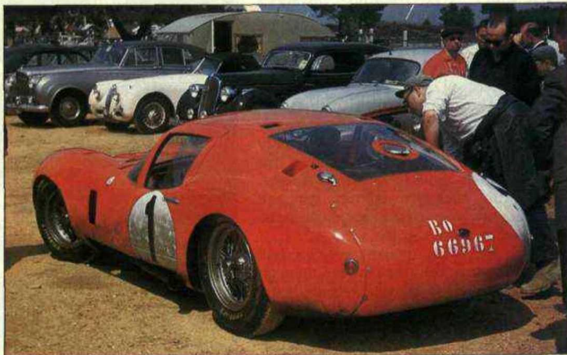
Frank Costin's careful streamlining was invalidated by careless execution of the Maserati's bodywork. Stirling Moss was slower on Mulsanne than the spyder.
