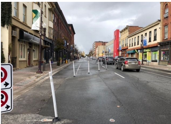
Figure 27. In some locations flexposts presented challenges in discerning directionality and depth of field.
