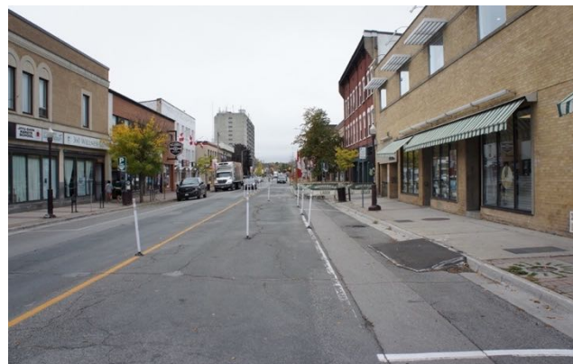
Figure 27. In some locations flexposts presented challenges in discerning directionality and depth of field.
