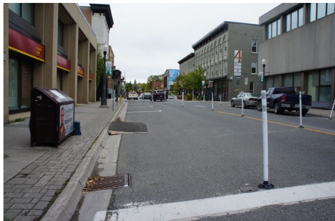
Figure 29. Expanded pedestrian space lacked visual cues indicating the space was for people.
