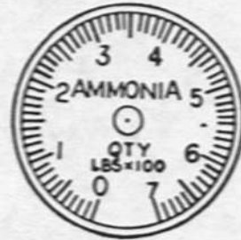
AMMONIA QUANTITY GAGE
