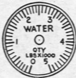
WATER QUANTITY GAGE
