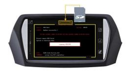
Once the home screen appears, connect the USB stick with the above mentioned files to the USB socket of vehicle
