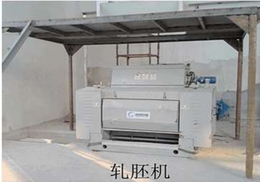
Oilseed Flaking Machine Slag Coveyor
