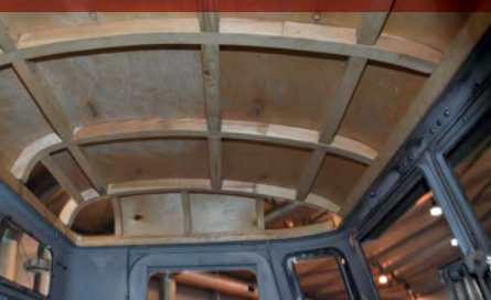
The cab roof was supported on a wooden framework, a common construction for Soviet military vehicles until the mid -1950s
