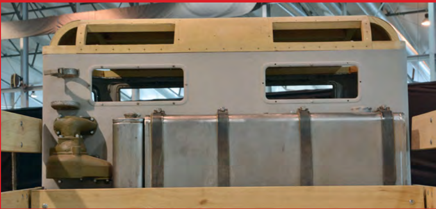
The STZ-5's fuel tank is mounted behind the cab in the cargo area
