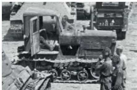
An STZ-3 in Red Army service. Note the all-steel road wheels and agricultural tracks
