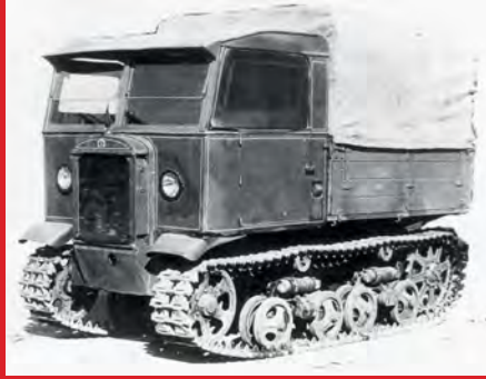
The early STZ-5 cab-over-engine artillery tractor prototype, with new road wheels and track
