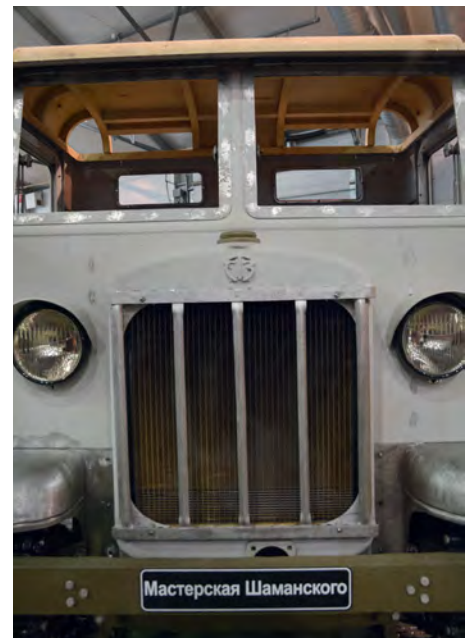
ABOVE: The STZ-5 has been completely rebuilt by the Shamansky Company, from a chassis and few recovered parts RIGHT: The STZ-5 has a distinctive cab and radiator, the latter bearing the STZ plant symbol
