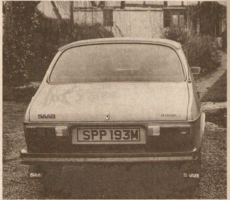
The bumpers are of the kind which can absorb low-speed shunts without damage and, usually, they do not ruin the cars appearance either.
