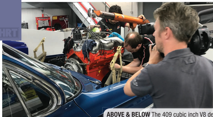
ABOVE & BELOW The 409 cubic inch V8 delivers 450 bhp and 450 lb/ft of torque – not bad for a car now almost 60 years old. The installation was surprisingly straightforward
