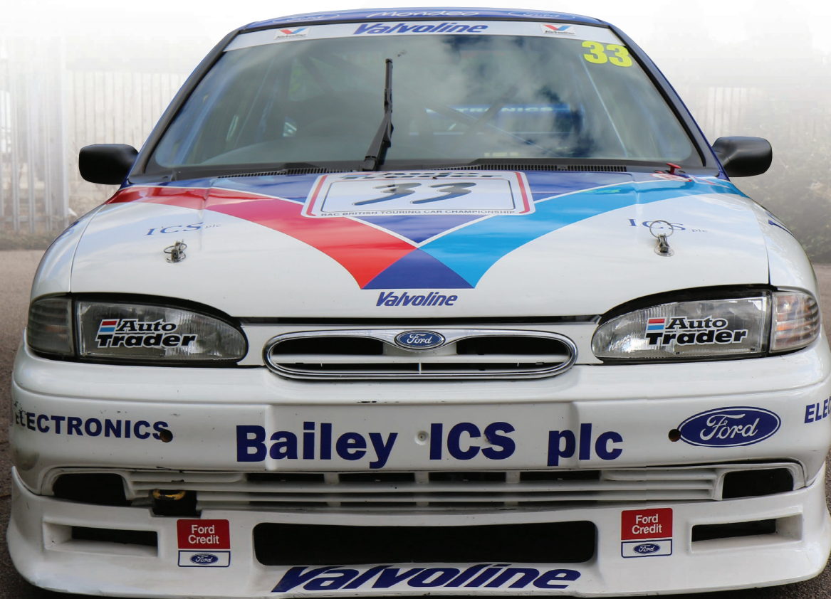
ABOVE In spite of the exotic nature of the Super Tourers, the front splitter and rear wing are the only composite parts visible externally
