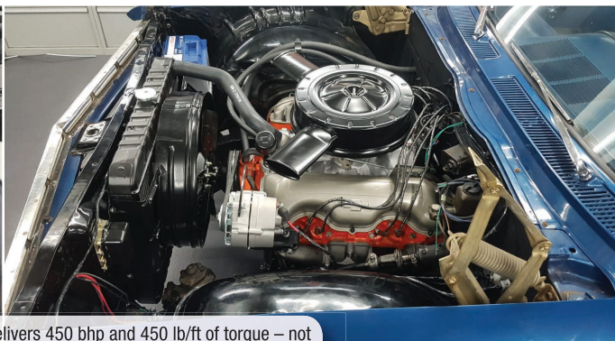
ABOVE & BELOW The 409 cubic inch V8 delivers 450 bhp and 450 lb/ft of torque – not bad for a car now almost 60 years old. The installation was surprisingly straightforward
