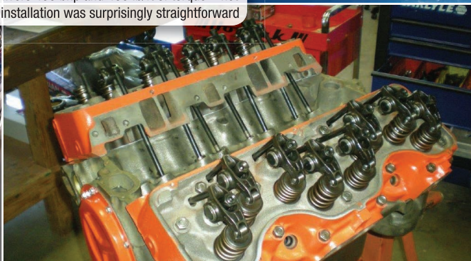
ABOVE & BELOW The 409 cubic inch V8 delivers 450 bhp and 450 lb/ft of torque – not bad for a car now almost 60 years old. The installation was surprisingly straightforward
