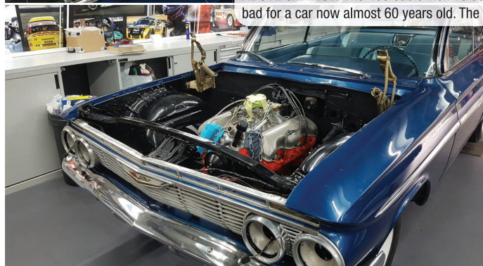
ABOVE & BELOW The 409 cubic inch V8 delivers 450 bhp and 450 lb/ft of torque – not bad for a car now almost 60 years old. The installation was surprisingly straightforward
