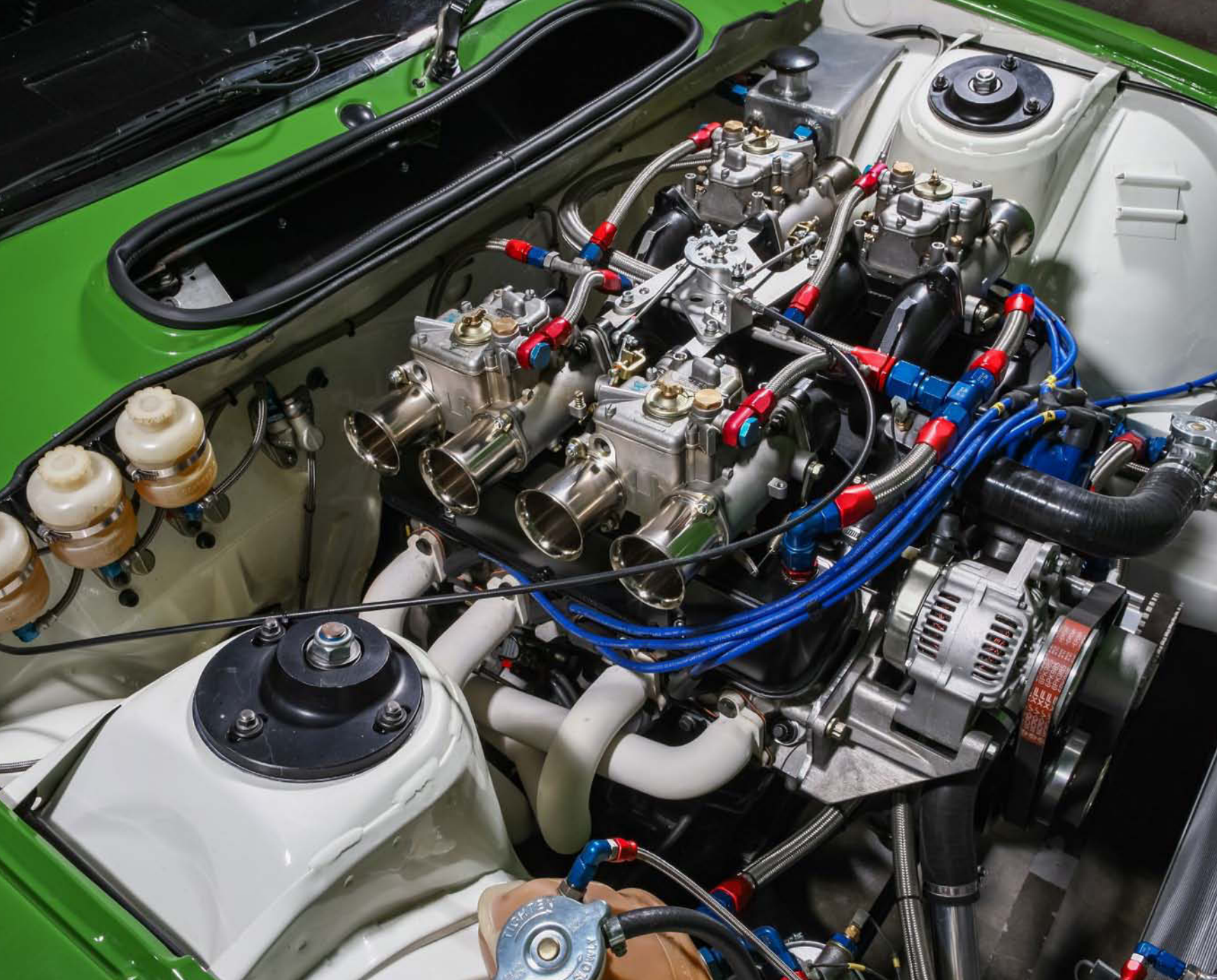
Beefier, brawnier and more of a racer, the Gp2 car with its four twin Webers has a wonderful voice, but it's tougher to hustle
