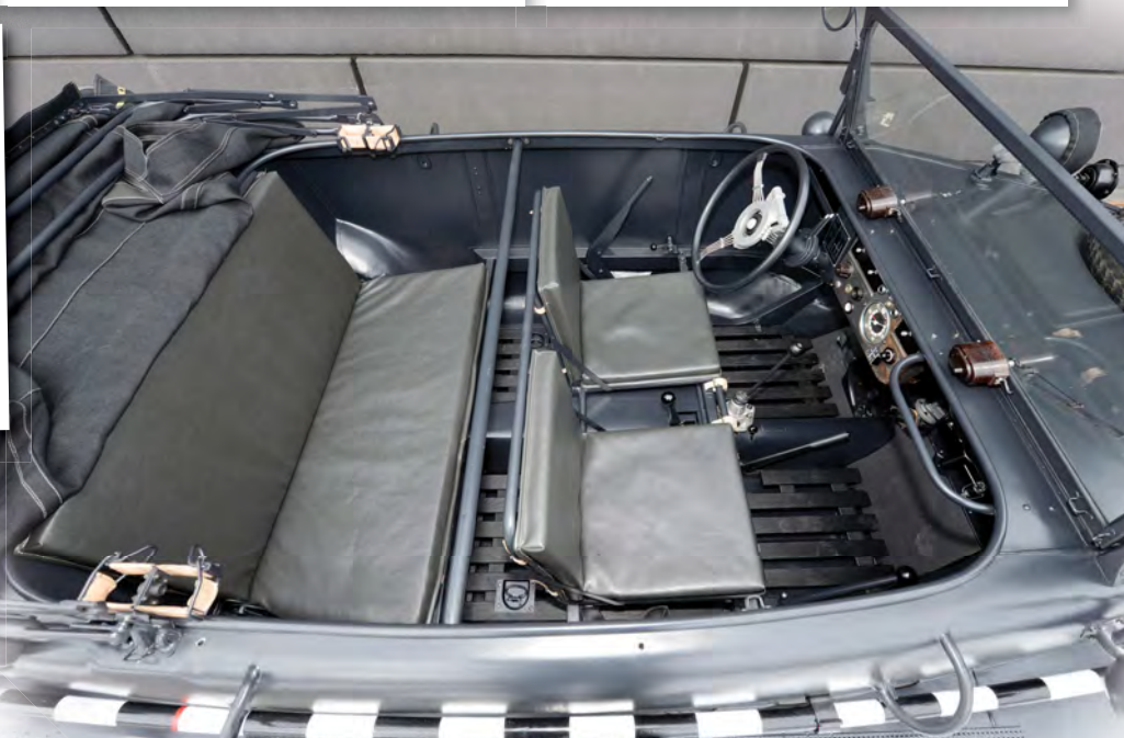
Above: A hinging steering wheel on 30 pre-series cars made it easier to get in and out. Right: There was significantly more space for the crew inside a Type 128 and the addition of a rear seat bench meant it could seat five in relative comfort.
