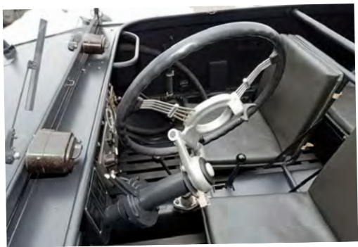
Above: A hinging steering wheel on 30 pre-series cars made it easier to get in and out. Right: There was significantly more space for the crew inside a Type 128 and the addition of a rear seat bench meant it could seat five in relative comfort.
