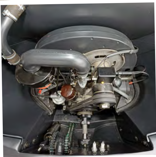
1132cc 25bhp engine was taken from VW's KdF. Note the drive for the propeller taken off the bottom pulley and the high position of the air intake so it didn't suck in water.
