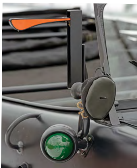
The green light on the starboard and a semaphore were standard items on the Type 128.
