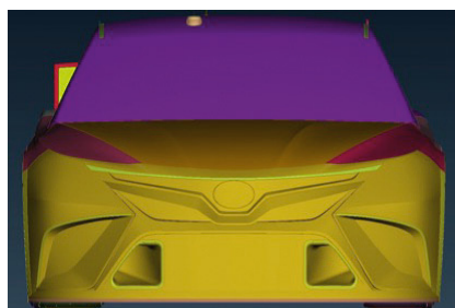
Toyota Camry Cup car CFD model with the aero duct inlet visible. This is also the brake duct inlet
