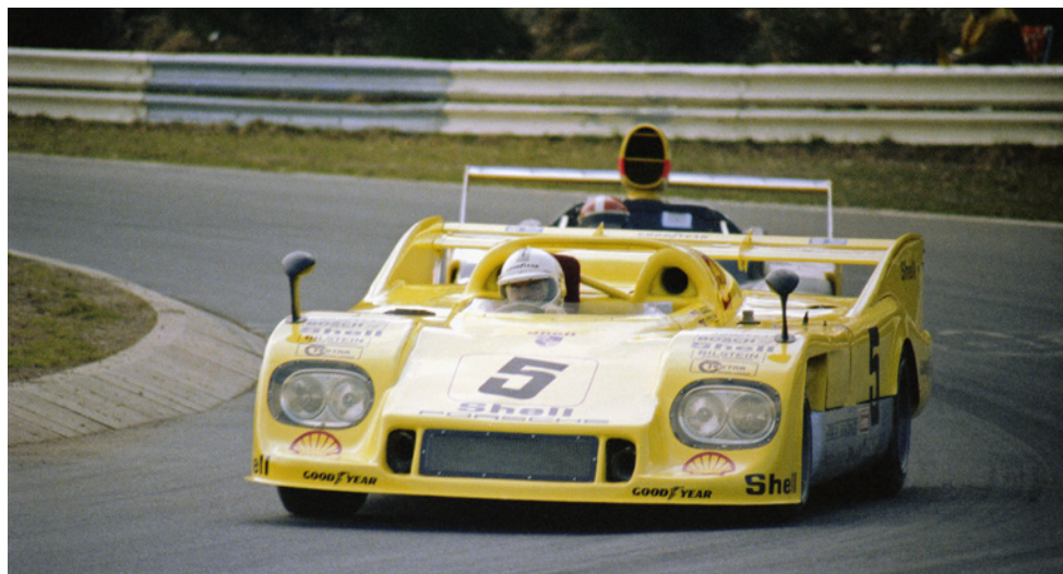
Porsche built the 936 as a works entry for the 1976 World Sportscar Championship but it was Joest and 908/03 chassis 008 that won the first round at the Nurburgring. Note the new 917/30 body and the headlights, which are from an NSU road car
