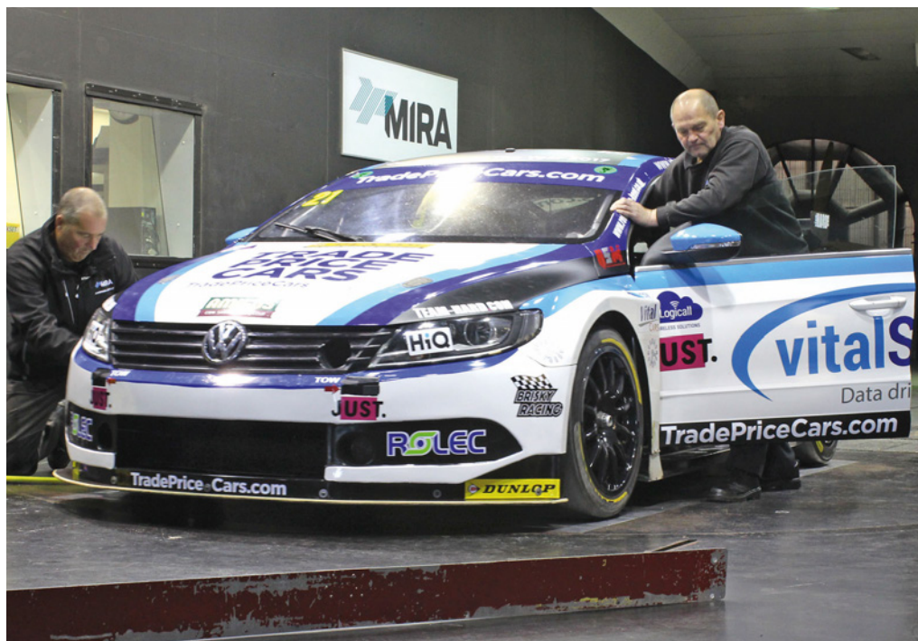
Setting up the Team Hard BTCC VW CC on the wind tunnel balance. The car has proved especially potent on fast circuits
