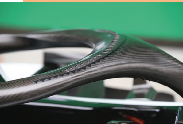
The the upper and lower edges of the Halo structure on the VF-18 are adorned with arrays of vortex generators
