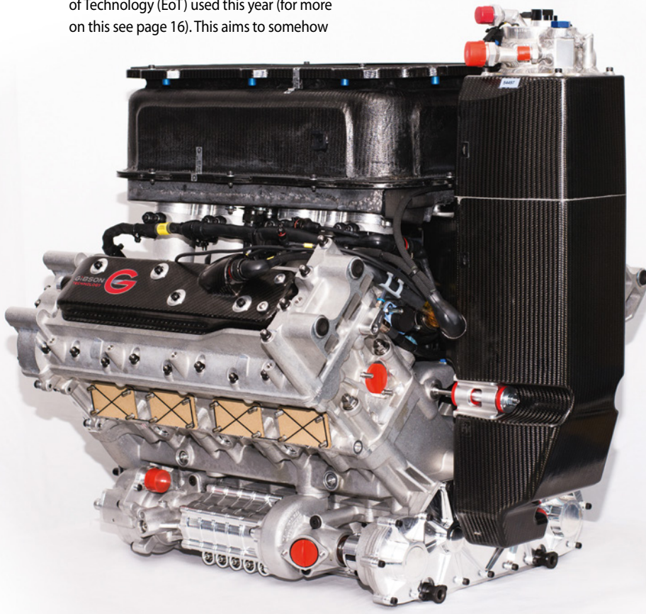
The Gibson (above) is the only naturally aspirated unit. Mecachrome has opted for single turbos, while AER and NISMO use a twin turbocharger layout. The Gibson is also the only one of the four to use port injection rather than direct injection
