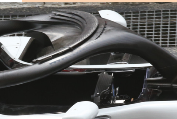
At the Spanish GP Haas experimented with winglets on the Halo, an approach that’s employed by most of its F1 rivals
