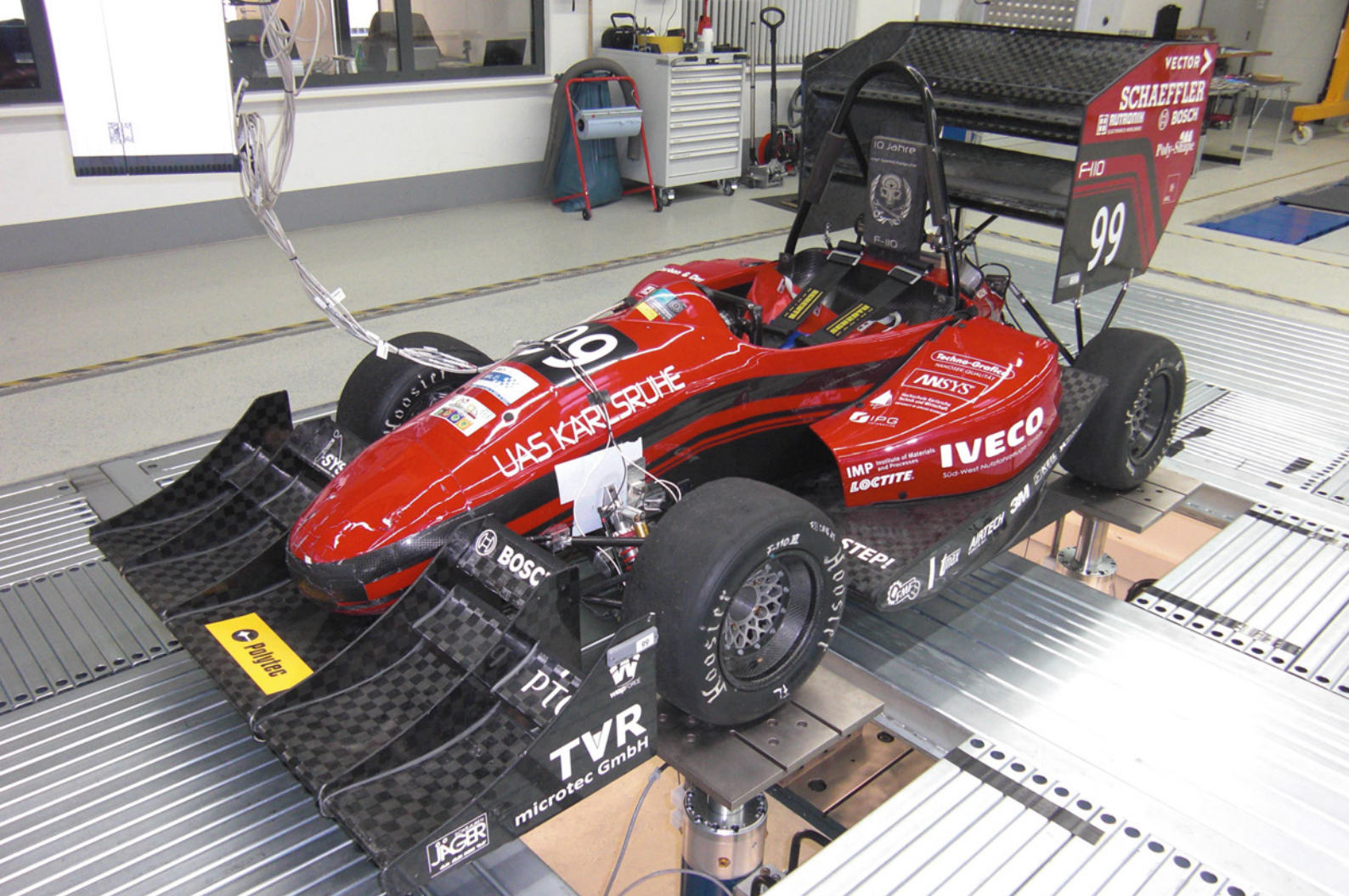
Four- and seven-post rigs tend to be adaptable and can be utilised to tune suspensions for pretty much any vehicle; whether it's a Formula Student (pictured) or a Formula 1 car
