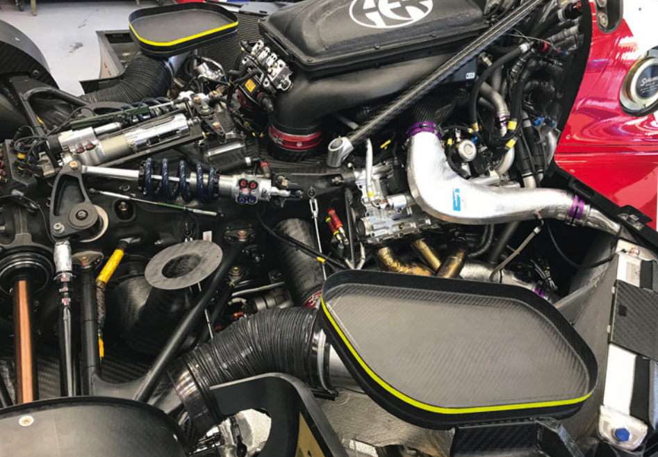
This season's twin turbo P60B engine from AER is based on the company's original P60 concept, which was last used in the WEC back in 2016 and was specifically designed to exploit the fuel flow restrictions of LMP1
