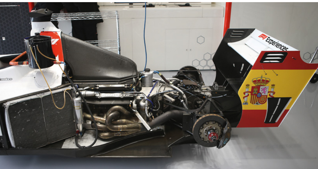
The European V10 powerplant started life as the Ford Cosworth VJ, the engine that propelled the Stewart-Ford in 1997/98
