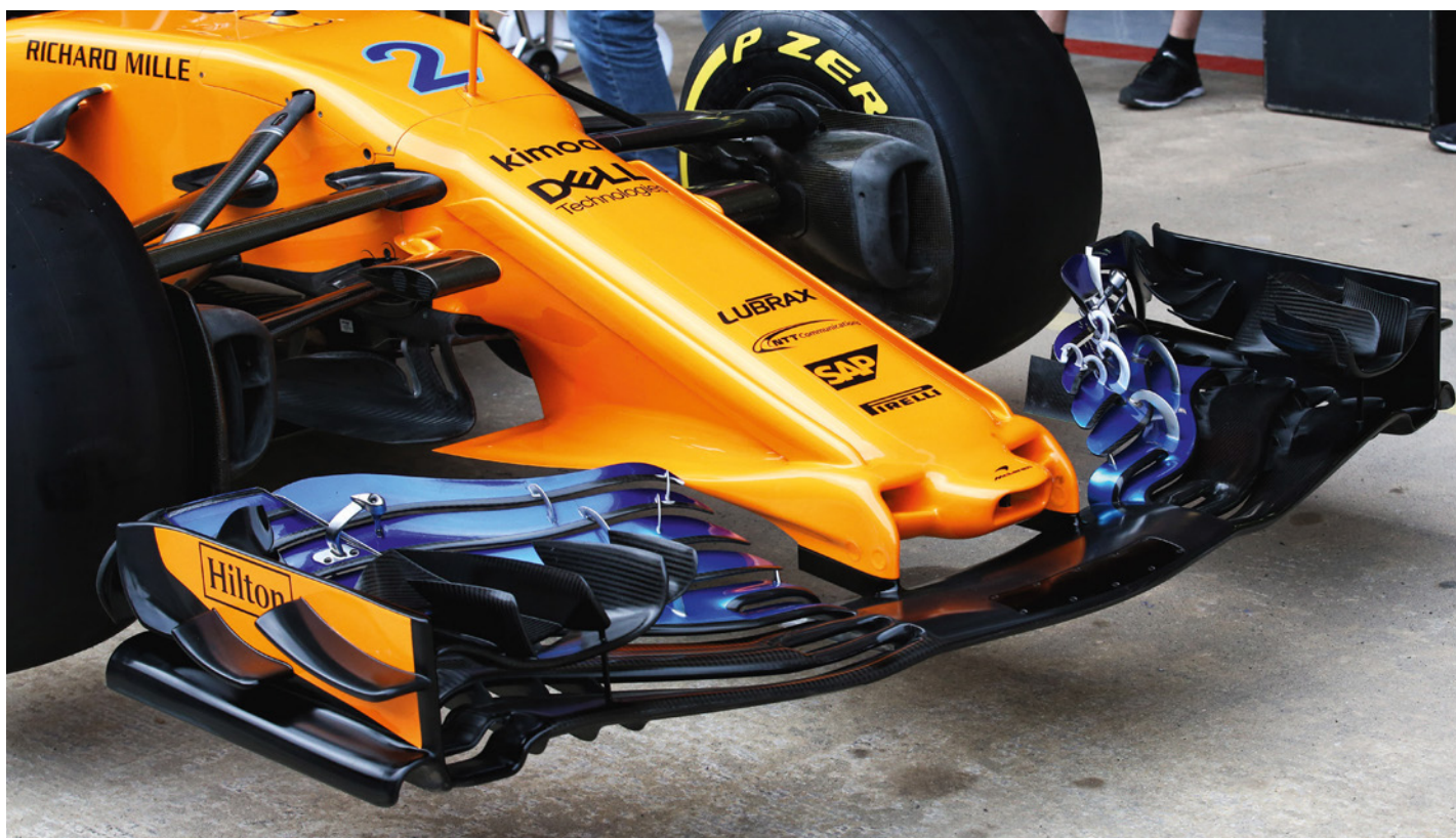
The highly complex front wings are the chief focus of the aero changes. The end plates and the top profiles will be shorn of the winglets and vertical fins that are now common in F1
