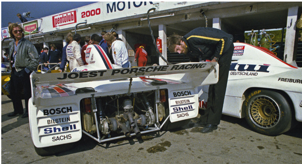
The business end of the last evolution of 008. The 630bhp twin-turbocharger Typ 935/73 engine made the 908/03 a difficult car to beat at any level. Its final full campaign was in the DRM series in 1982, then a safe haven for obsolete Group 6 cars
