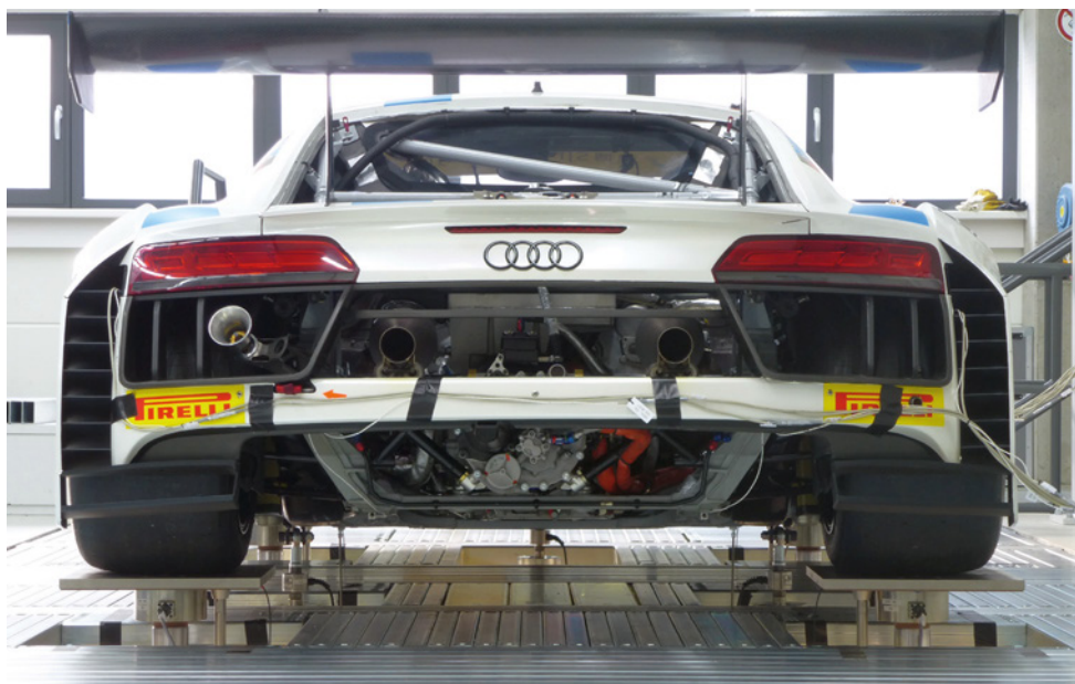
At each corner wheelpan actuators drive displacements into the wheels to simulate track inputs. There are also the three aeroloader actuators which emulate the effect of downforce; usually with one at the front and two at the rear, as seen here
