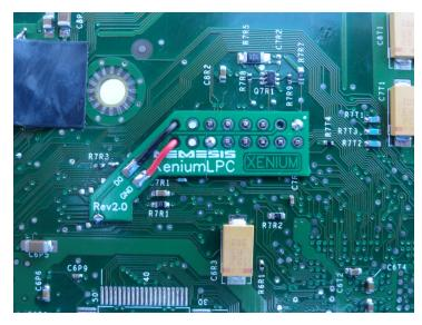
Even without serving much purpose it does look good when installed. It's not necessary to solder every pin, just the ground marked with the white dot. I did the opposite pin to hold it in place better and made a nice bead over the D0 on the motherboard.
