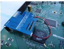
And finally after having cleaned up the wires and solder from a previous attempt at a LPC rebuild. Then having installed the XeniumLPC for v1.6, this is what a "Pin Header" installation should look like on version 1.6 and 1.6b consoles...
