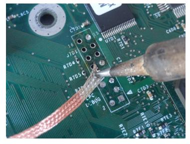
Put the tip of the Wick on top of the through hole and with the soldering iron set to 360°C press down on the Wick. You will notice the solder move up the Wick, when it stops remove the Wick and soldering iron. Cut off the Wick that's soaked in solder and repeat the process.
