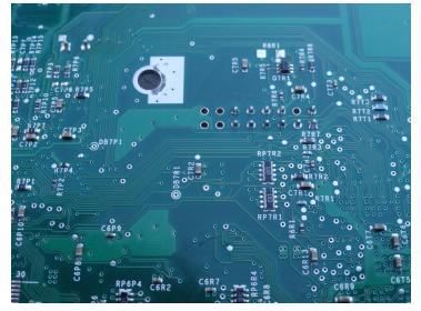
I decided to clean this up and prepare it for a XeniumLPC rebuild for version 1.6 consoles. Started by removing all the wires then applied flux to all the area's that had been soldered. Using wick I went around and desoldered all the pads and removed most of the solder from the Pin Header. I resoldered the Pin Header using flux at 360°C making sure the solder went into the holes.
