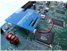
I continued to use the version 1.0 console that I did the desolder on, for the images used within this installation guide. And this is what a "Pin Header" installation should look like on console versions 1.0 through to v1.5...
