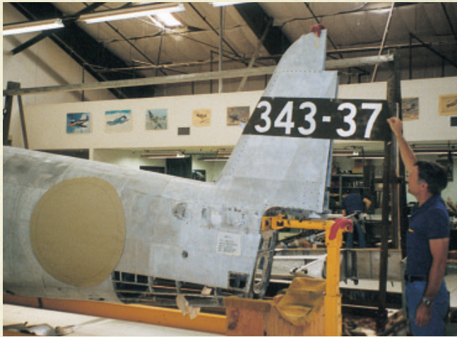
When the Champlin Museum restored the "George," many of the internal components were missing; if an original part could not be located and reinstalled, it was remanufactured (photos by Robert Mikesh).
