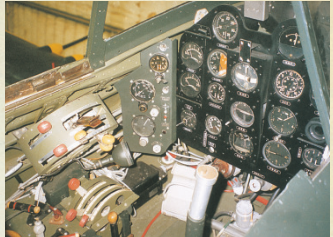
When the Champlin Museum restored the "George," many of the internal components were missing; if an original part could not be located and reinstalled, it was remanufactured (photos by Robert Mikesh).
