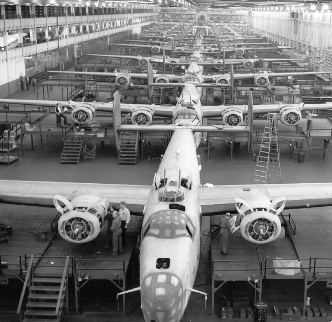
LIBERATOR LINEUP B-24s on the assembly line at Ford's Willow Run plant in Michigan, one of five factories that cranked out the bombers.
