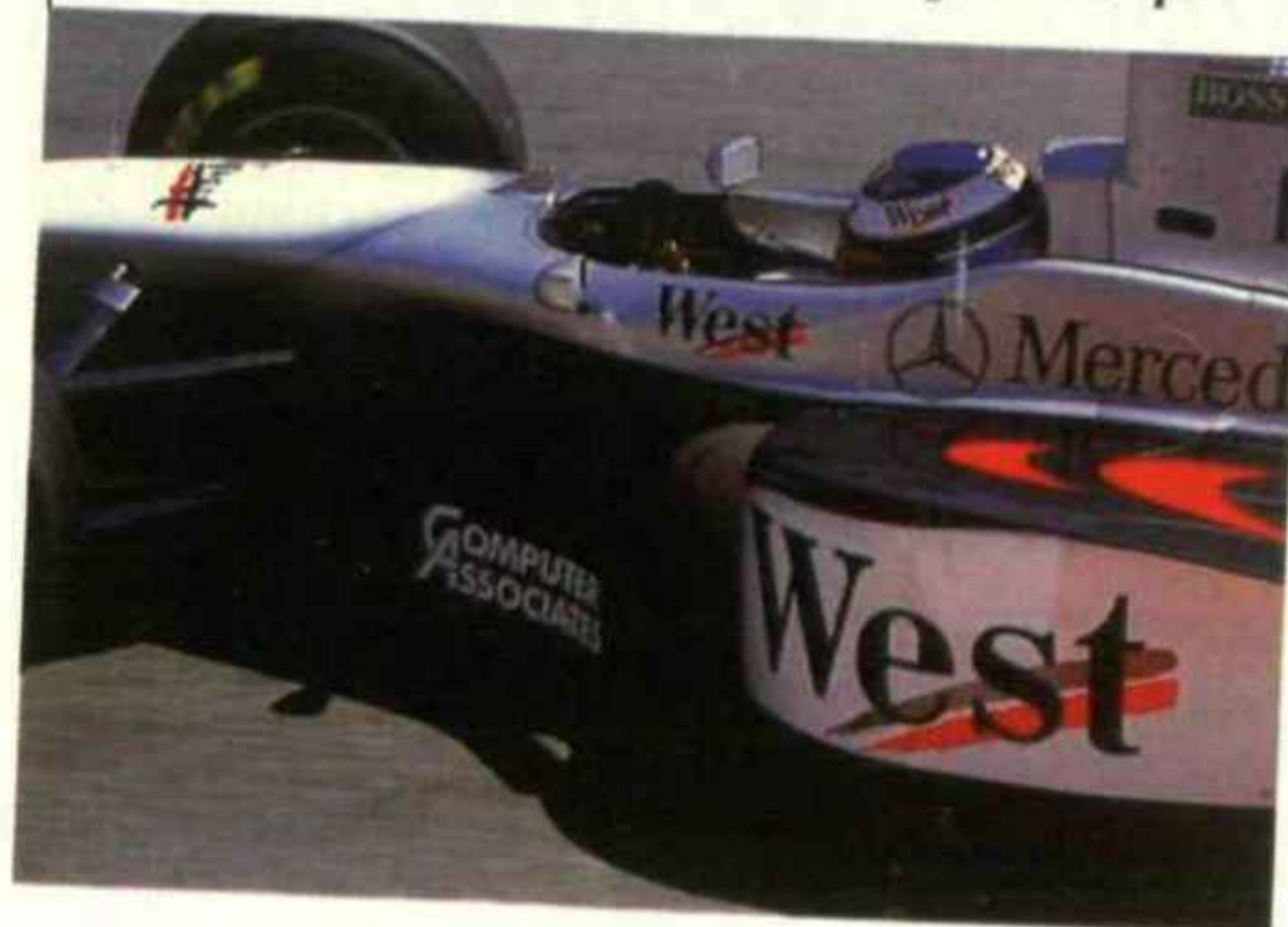
Below: 1997; Hakkinen's McLaren MP4/12 during Hungarian GP. Note how his head is protected not just by his helmet but also the sides of the cockpit
