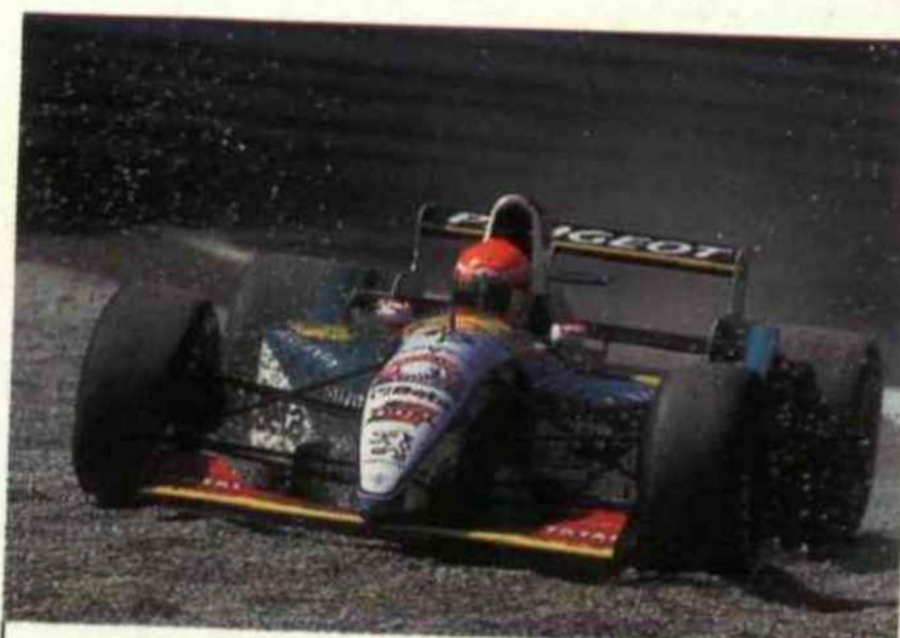
Above: 1995; Eddie Irvine's Jordan 195 buried deep in the Monza gravel. The gravel trap replaced catch fencing as the decelerator of choice for out of control F1 cars. Used properly, it is devastatingly effective.
