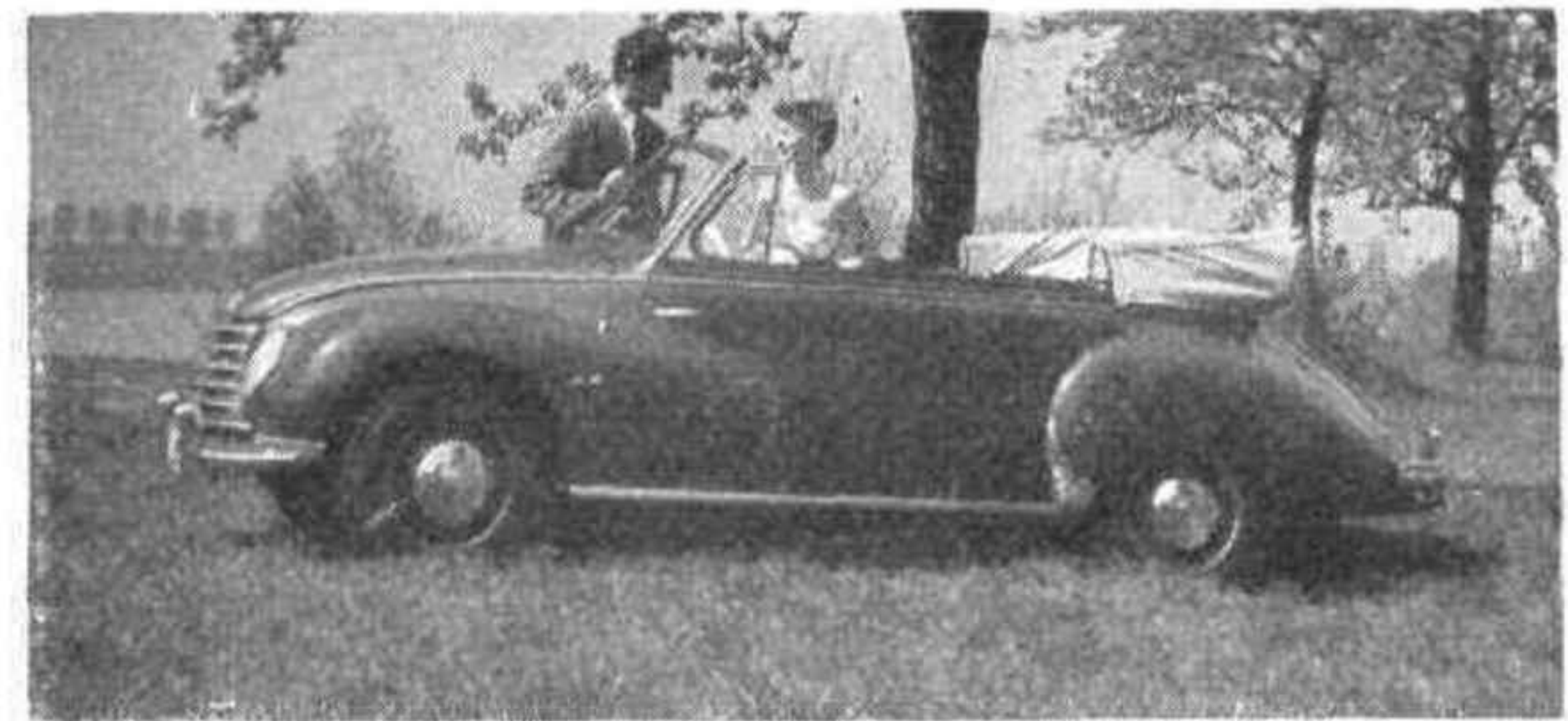
THREE-CYLINDER TWO-STROKE.—The new D.K.W., said to give extremely good economy with a maximum speed of about 78 m.p.h. in five-seater saloon form.
