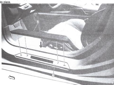
8. Close the door for one minute and then open the door and ensure accessory sill trim plate (1) illuminates.
