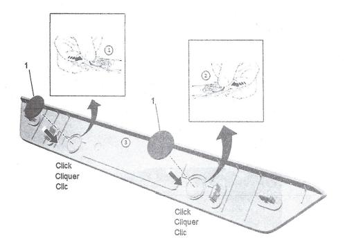
7. Align the clips of the sill trim plate (2) over the attachment holes on rocker sill (1) and firmly push down on the sill trim plate (2) until it snaps into place.
