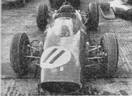
brakes are mounted inboard. Most important, magnesium alloy knock-on wheels are now featured.
