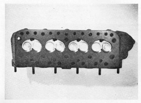
STAGE 1 Janspeed cylinder head for a Mini-Minor (above).
