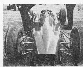
THE REAR END of the Ferrari is by double wishbones. The light alloy hub carriers extend close to the road in a Lotus-like manner.
