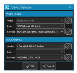
Here it is possible to set up the current device parameters. The Settings buttons here (with spanner icon) open properties for DirectShow devices (like web-cameras). By setting required format, input stream is received:
