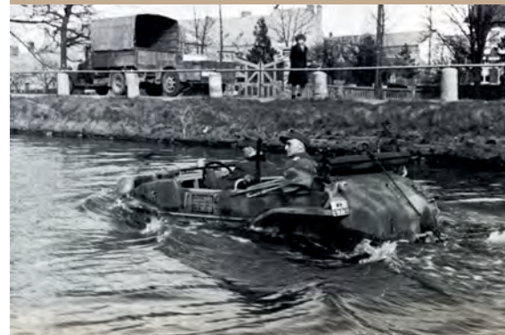
Carrying only two soldiers, a Schwimmwagen's freeboard was more than adequate as it cruised down a French canal. Strong bow waves suggest that it was running at its maximum speed in water of 5½ knots
