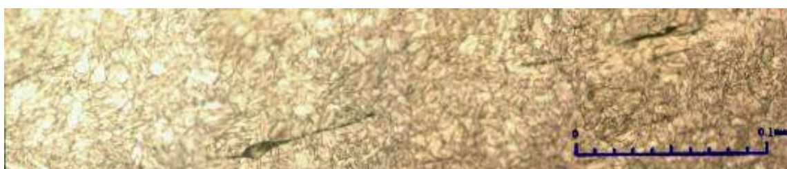
Figure 3. Sulphides, sample CM8R, hot processing, magnification 500xs
