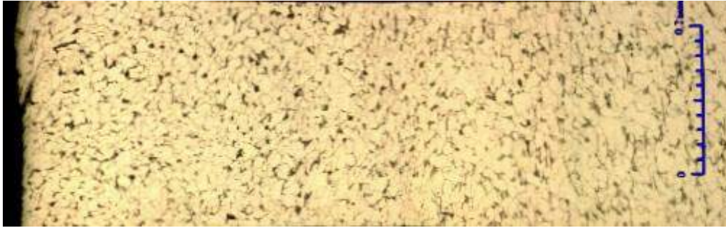
Figure 4. Sample CL8R and ferrite – pearlite structure, magnification 500 xs
