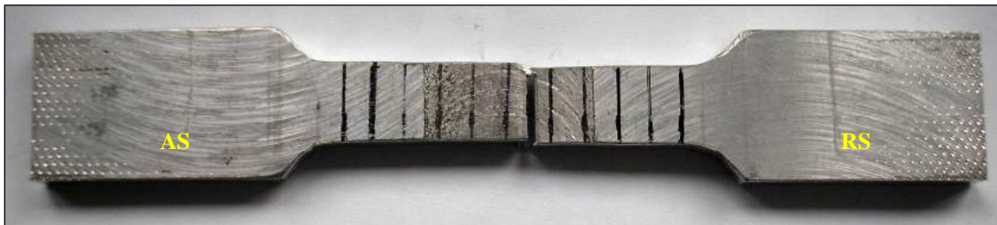
Figure 7. Pulled specimen after failure [5]
