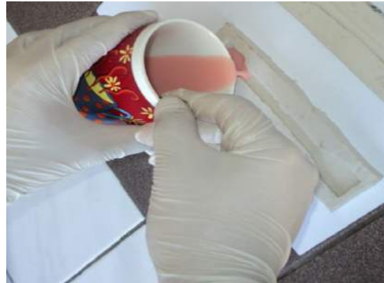
Figure 5. Pouring the polymer into a mold.
