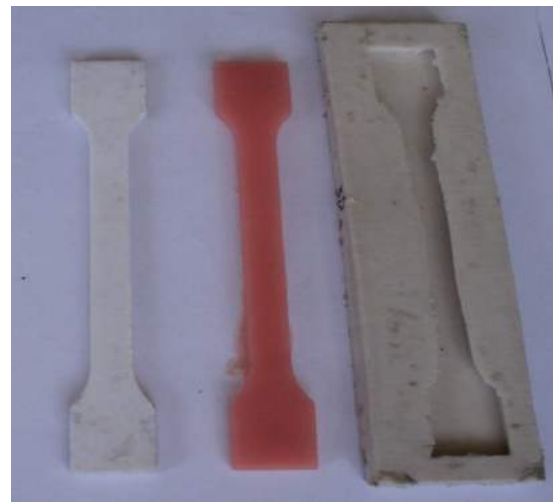
Figure 7. The physical model, the part and the mould
