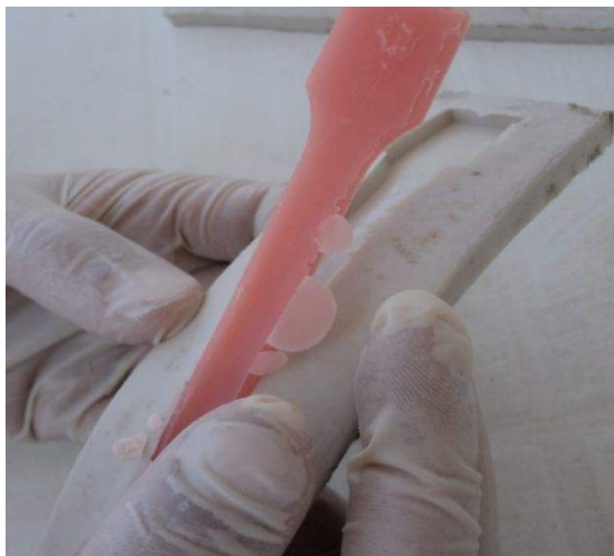
Figure 6. Removing the part from the mould
