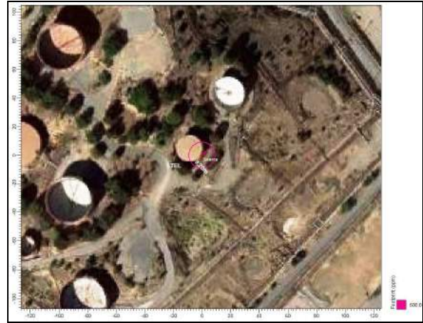
Figure 8. Footprint layout, Risk contours for 600 ppm. Downwind distances: STEL = 9.20 m
