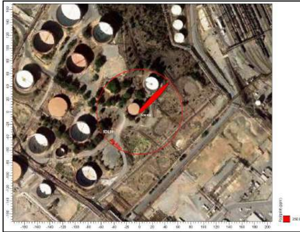
Figure 7. Footprint layout, Risk contours for 250 ppm. Downwind distances: IDLH = 66.80 m
