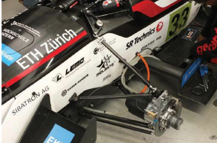
Gotthard's four hub-mounted electric motors deliver 54 horsepower and they weigh a paltry 3.4kg. The motors were redesigned for this year and now produce more power
