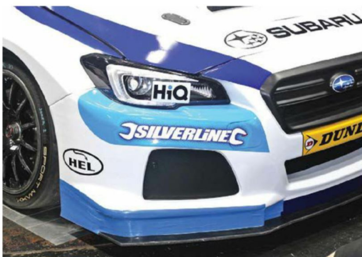
A further small drag gain was achieved by filling in most of the transverse undercut
