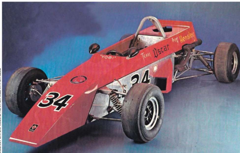
The first Xpit with original bodywork. It used a simple chassis frame made up mostly of square-section mild steel tubing
