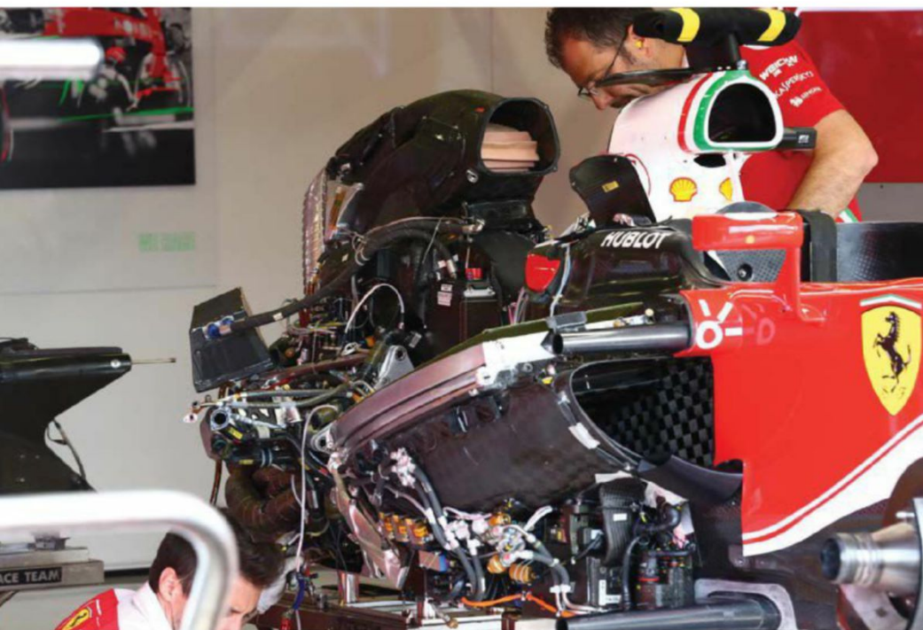
The VF-16 shares much of its engine installation and cooling philosophy with the Ferrari SF16-H (pictured). This is not really surprising as Haas buys most of its components from the Scuderia. Its links with Ferrari caused controversy last season
