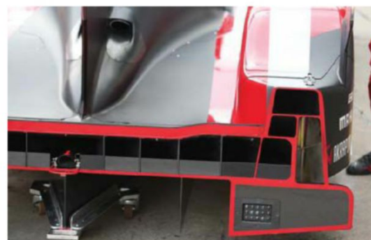
Audi revised its cooling layout for the second half of the WEC. The rear exit of the bodywork was modified with a number of segments added to the Spec C (below right) used at the 'Ring. Spec A (above left) was used at Silverstone only, the similar but lower drag Spec B (above right) car was used at Spa and Le Mans
