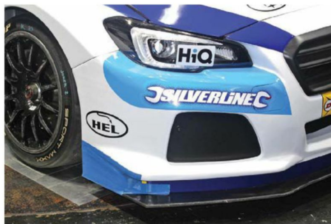
Filling the outboard scallop on the Levorg achieved nearly half of the drag benefit found by smoothing out the bumper – as well as all of the modest downforce loss
