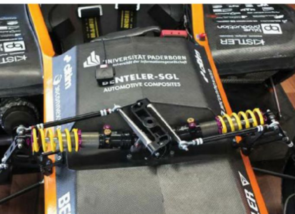
Paderborn used purpose-made Formula Student dampers from KW Suspension. The pair of dampers are mounted horizontally on the top of the chassis – note the neat linkage between them
