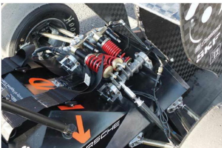
Renstall Esslingen used a triple damper layout at the rear, the third to support aero, in common with a number of 2016 cars – but it used a different concept with the pitch and roll separated
