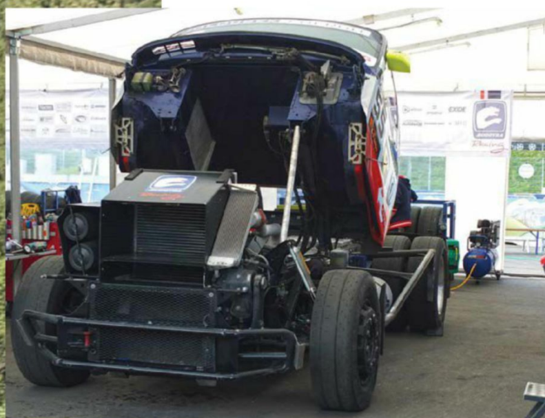
The Buggyra 'cab rear' style Freightliner truck with its bodywork removed. The bump bar at the front of the chassis gives an indication of just how physical FIA European Truck Racing gets
