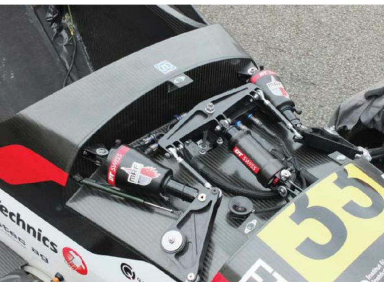
The car features a three-element suspension with a heave spring for the aero loads. Single-wheel springs feature magnetorheological technology for adjustment on track
