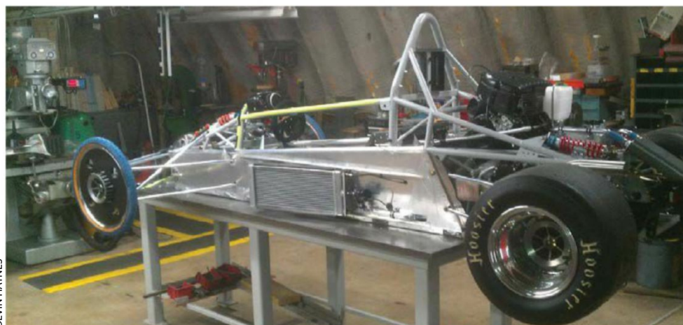
Morton's stretched Gamma II near completion. The car's wheelbase is now at 92in and front and rear tracks are 54.5in and 50in respectively. The plywood training wheels on the front are an essential addition in order to fit the racecar into the trailer
