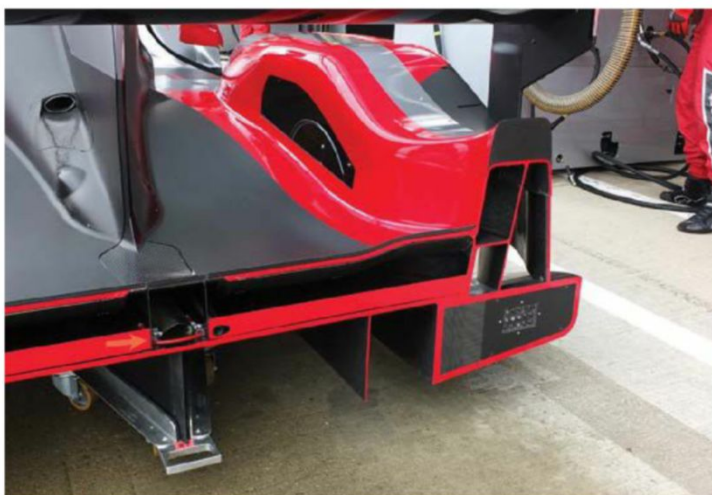
Audi revised its cooling layout for the second half of the WEC. The rear exit of the bodywork was modified with a number of segments added to the Spec C (below right) used at the 'Ring. Spec A (above left) was used at Silverstone only, the similar but lower drag Spec B (above right) car was used at Spa and Le Mans
