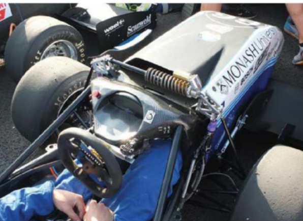
The Australian Monash entry caused quite a stir in the Formula Student paddock. Its suspension set-up has been described by the team as a hydraulically actuated mode separated system
