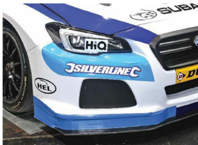
Further smoothing of infill below the lower inlet achieved another small drag benefit
