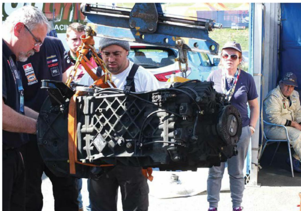
Racing trucks must use a production gearbox with the standard amount of available ratios. This means that there can be as many as 16 gears, but because of the huge amounts of torque (some 5500Nm) drivers tend to use just two or three in a race
