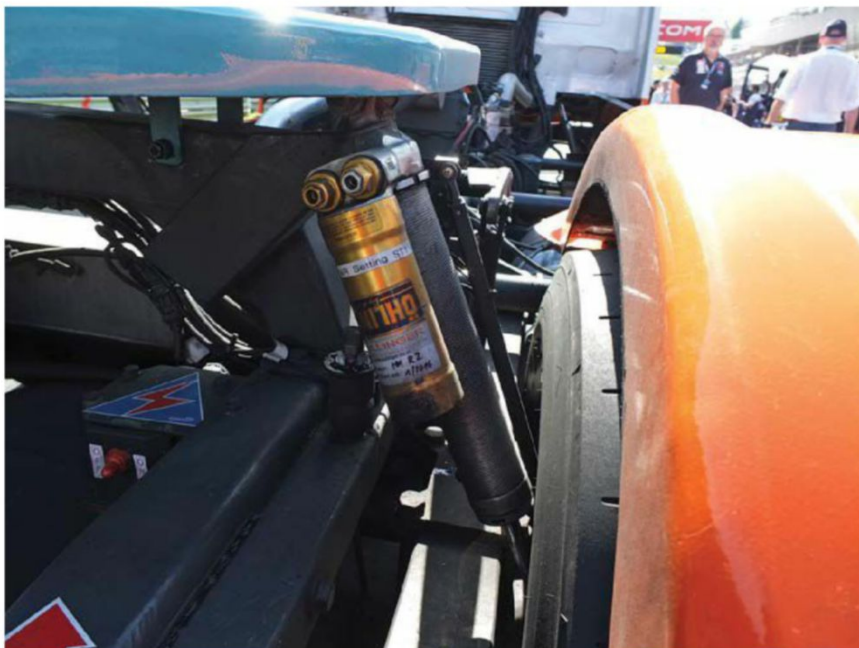
A whopping Ohlins TTX damper on a MAN race truck. Damper development is a vital part of race truck engineering as the spring rates run by the trucks are generally quite soft. Motorsport shocks are used
