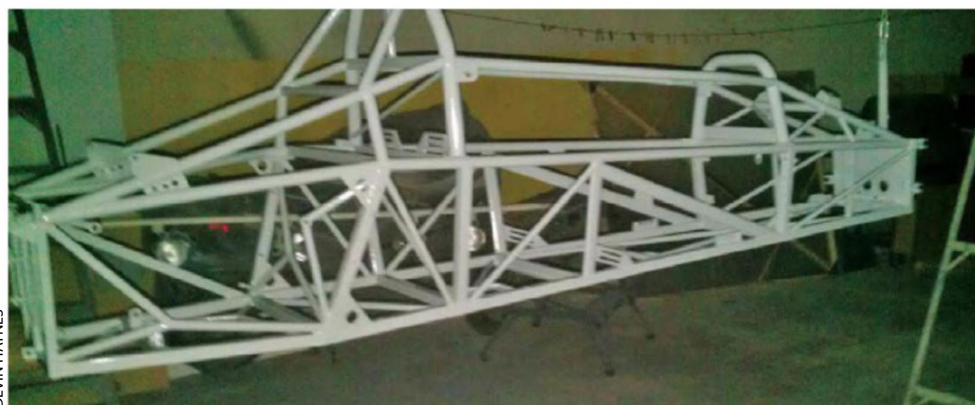
Stretched Gamma II frame after powder coating. The modification was made because Morton needs more space in the car
