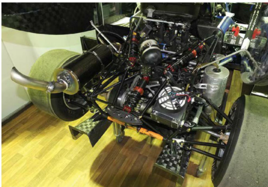
The gigantic rear wing assembly on the F0711-11 sits atop a Yamaha YZF-R6 499cc in-line four engine. Note the third element suspension, with its heave spring to support the racecar's ambitious aerodynamic package
