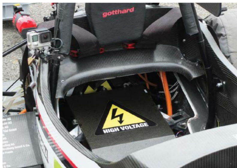
Half of the split battery pack; the other half goes under the driver's legs, which has enabled the team to construct a completely new undertray while also lowering C of G
