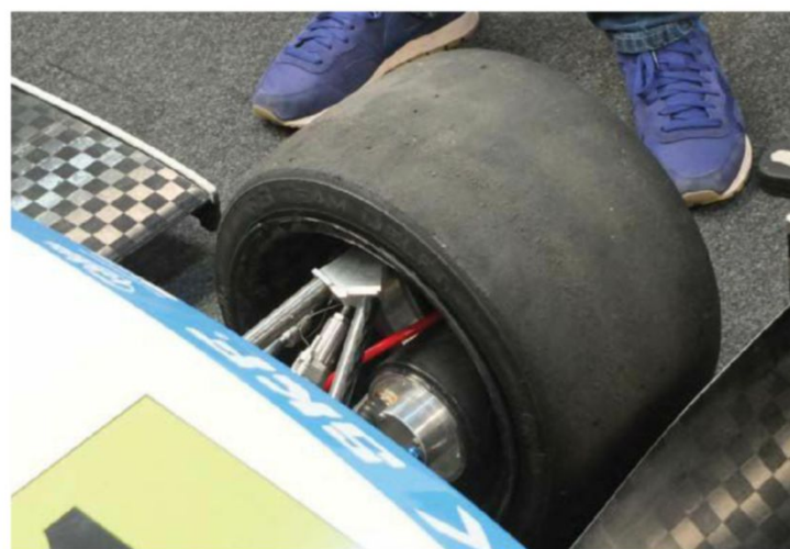
Hub motors and small wheels made the suspension mounting tricky for defending champ team Delft. Its other main focus was stiffening the car's suspension with carbon fibre rods
