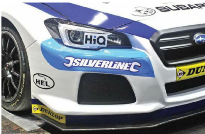
The baseline airdam was designed purely from previous experience. It featured an undercut across the whole of the splitter and an inset scallop in front of the wheel
