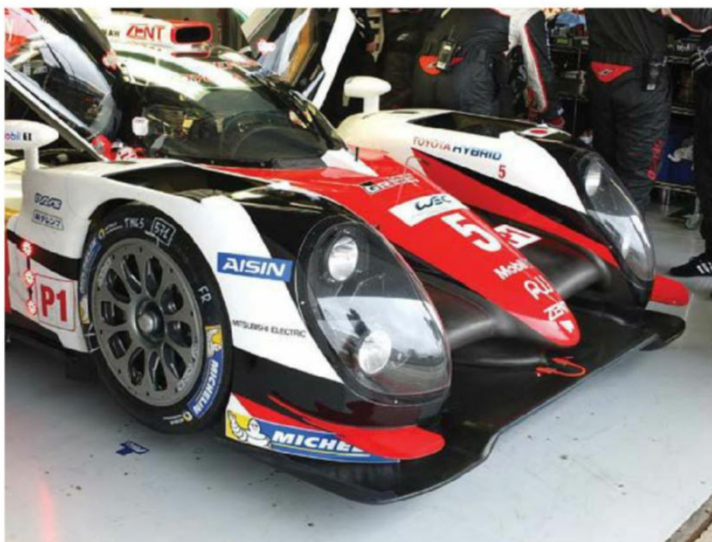
The new Spec C aero kits were aired at the Nurburgring for the first time this season. Toyota revised the front end of the TS050 for the latter part of the WEC, using the Spec A version (above left) of the body seen at Silverstone and Spa as a basis. The Spec C version (above right) features new, longer, flatter front dive planes in place of the bat-wing style of Spec A
