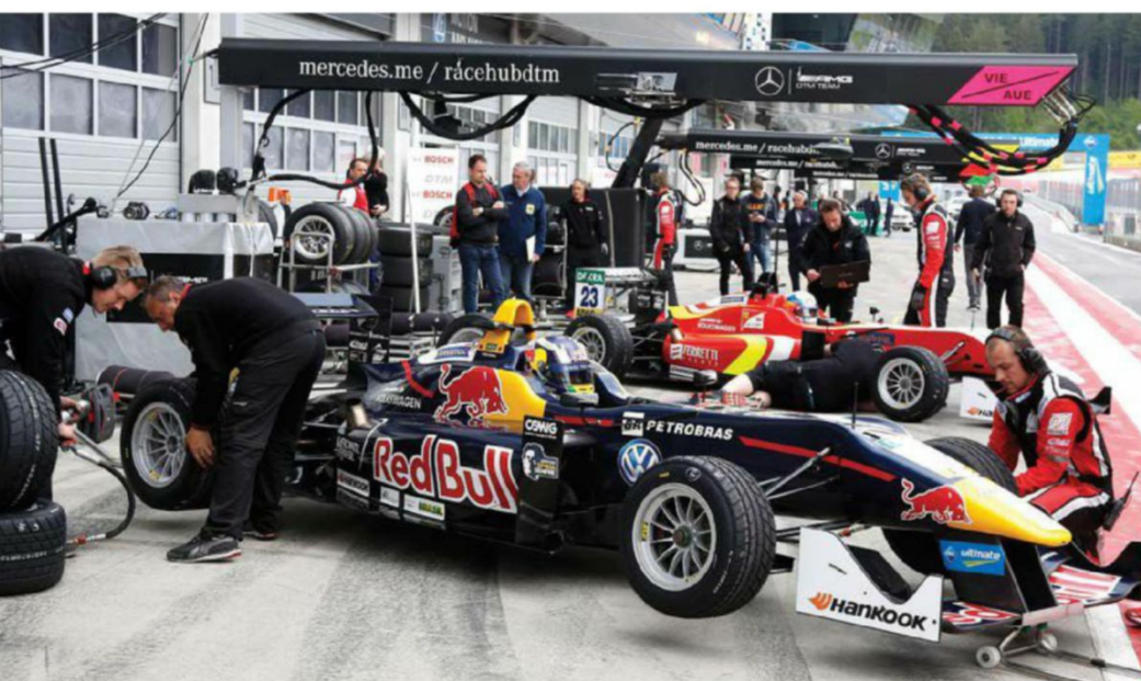
The elegant Dallara chassis has proved itself to be robust in a number of high profile shunts in recent seasons yet there is still a real possibility that in the future F3 cars might be required to run with Halo or some other form of cockpit protection
