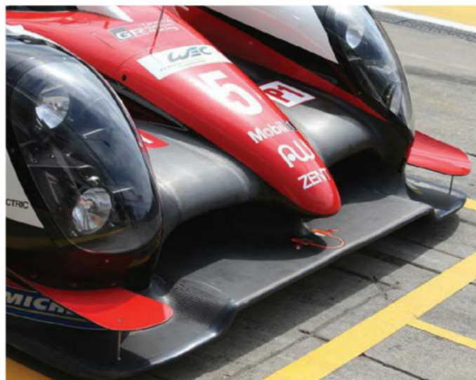
The new Spec C aero kits were aired at the Nurburgring for the first time this season. Toyota revised the front end of the TS050 for the latter part of the WEC, using the Spec A version (above left) of the body seen at Silverstone and Spa as a basis. The Spec C version (above right) features new, longer, flatter front dive planes in place of the bat-wing style of Spec A
