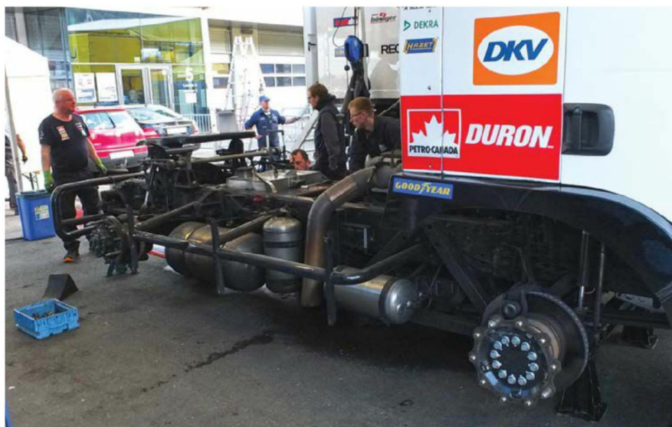
The brakes are water cooled in order to get them through a race of 20 to 25 minutes. There are two nozzles on the front brakes spraying water into the disc's air vents. Trucks use steel discs rather than carbon, for reasons of durability and price
