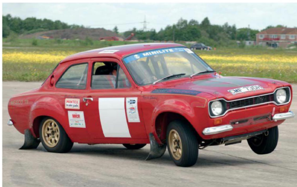
A fully unloaded inner wheel on a hard-pressed Ford Escort Mexico rally car – just one of the effects you can expect when an older-style steering system is put through its paces. The steering axis will move as each variable is changed
