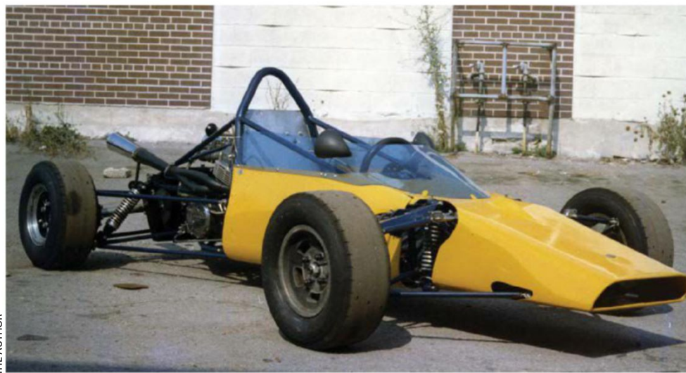
Luchinger F4, seen here after the installation of a Honda 750, was run with a turbocharger fitted when it was in 500cc guise
