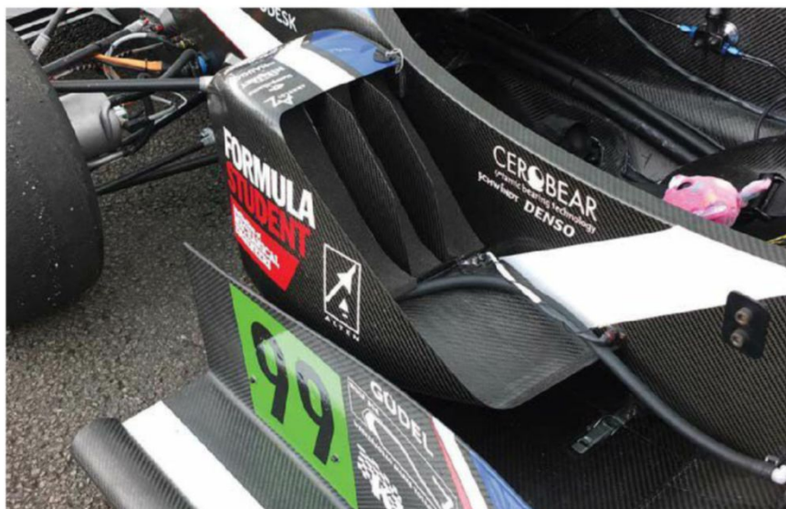
Aerodynamic detail reached new levels at this year's event, as this very neat sidepod ducting work on the RWTH Aachen entry shows. Cooling has also become a key battleground in Formula Student competition
