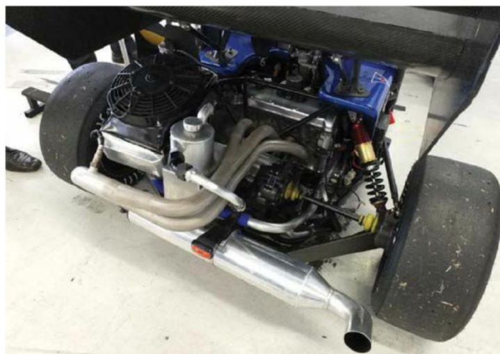
Edith Cowan University's car ran a De Dion rear beam suspension with satchell links so it didn't have to have a subframe on the rear. This allowed it to use a full-length monocoque
