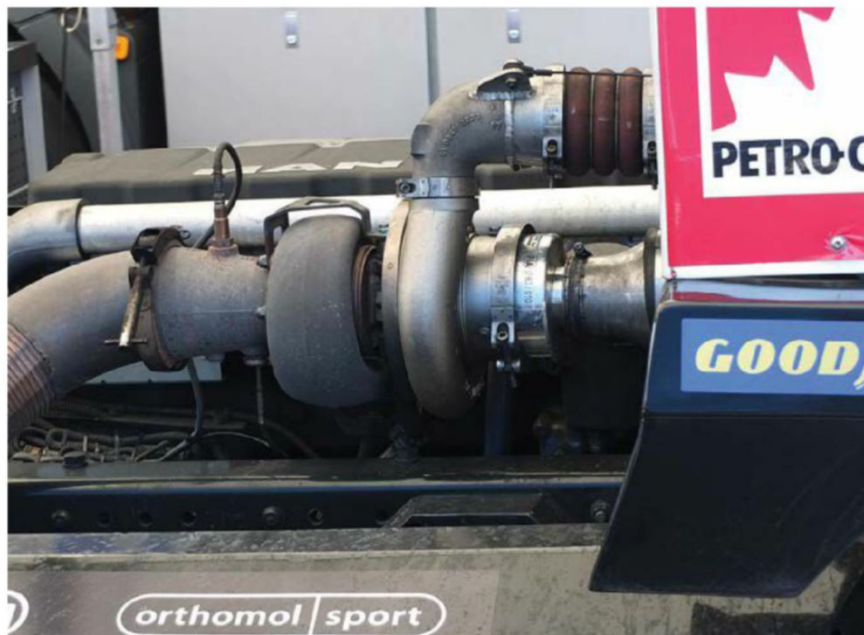
Turbochargers in truck racing tend to be on the large side. The teams spend a great deal of time in finding the sweet spot on their turbos, both by running the engine on the dyno and in straightline tests at airfields
