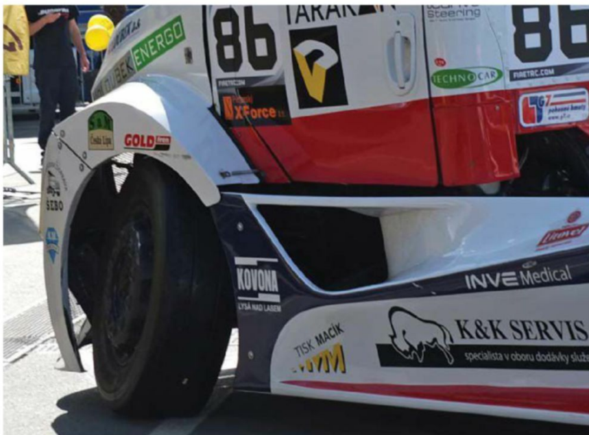
The trucks run up to 35 degrees of caster to increase the cornering speeds. They use hydraulic steering systems largely derived from production vehicles, using 400bar of pressure with these big caster angles
