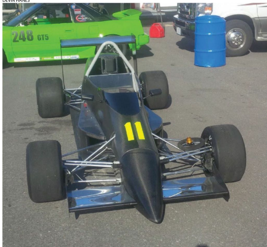
Jim Morton's Gamma II F4 with its new CFRP bodywork. This 750cc machine regularly mixes it with 2-litre cars
