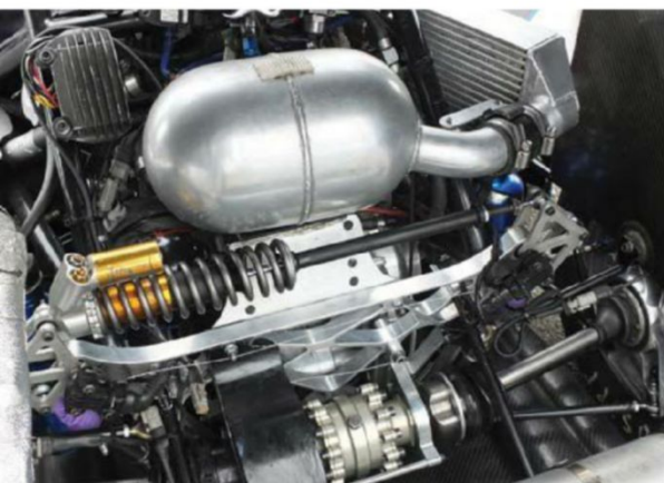
The rear of the Monash car. The aim of this ingenious system is to separate and isolate each type of chassis movement (roll, pitch, heave, bump and warp) so they can then be independently tuned
