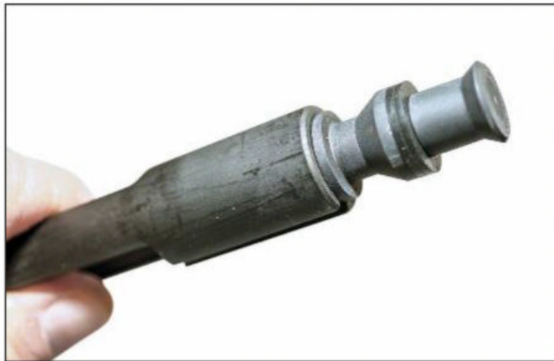
The carrier adapter is a press-fit into the rear of the assembled carrier.
