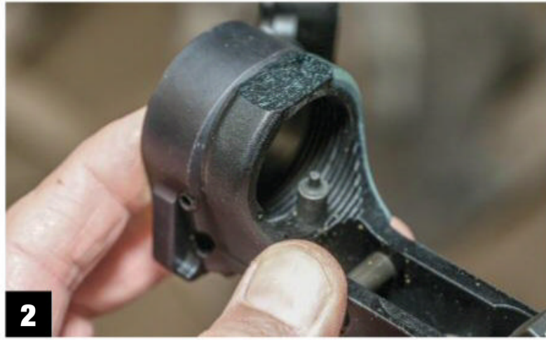
2 And then press the adapter to the receiver. Tighten the locking collar until you flex the wrench. (I bent mine, probably a bit too much, that.) Don't worry about the buffer retainer, it goes into the adapter later.
