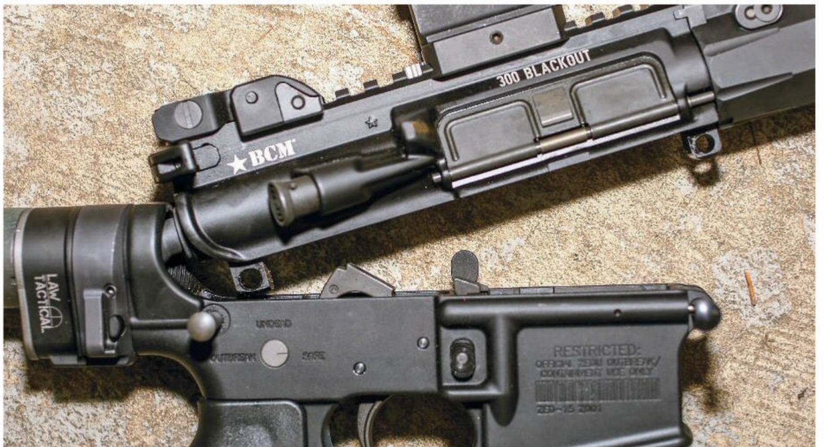
To take the folded pistol apart, you have to press both takedown pins through, and then lift the upper away from the lower. It won't hinge open.
