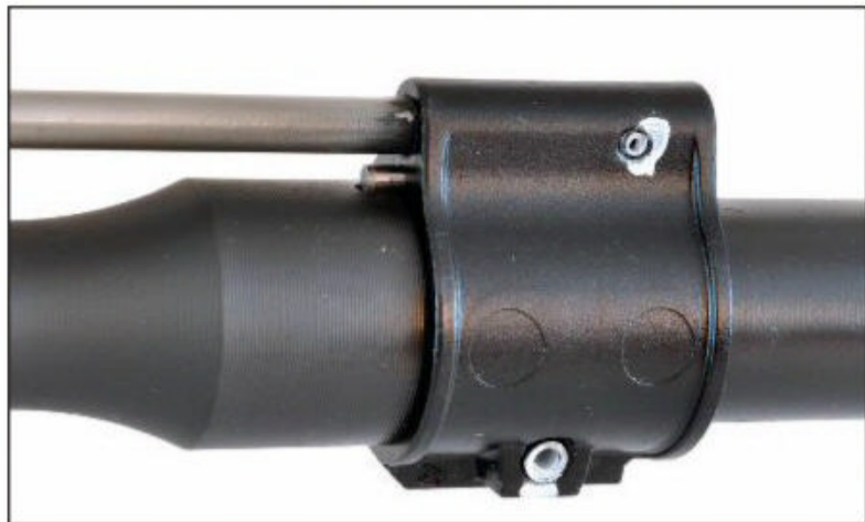
In the Super Duty rifle you'll see Geissele's stainless steel Super Gas Block which has a tiny indexing pin at the rear which fits into a slot they've machined into the top of the barrel for perfect alignment.
