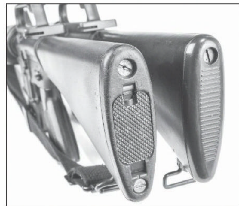
The early model solid buttstock is shown on the right. Later versions had a trapdoor storage compartment for a cleaning kit or a few emergency M&M's.
