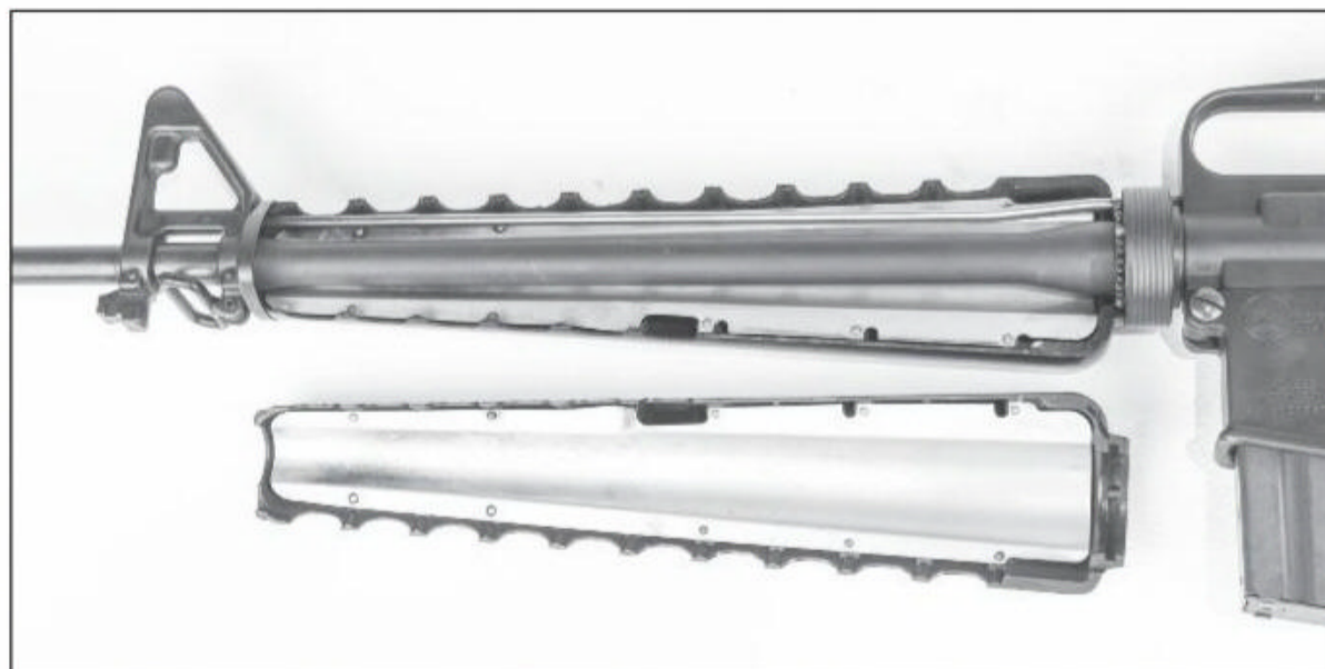
The modern direct gas impingement system all started here. The black plastic handguards sport aluminum heat shields and are unique to their respective sides of the rifle.
