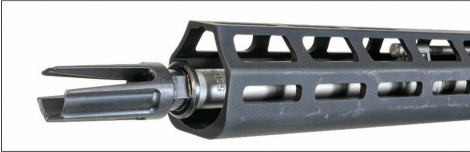
The medium-light contour stainless steel barrel has a 5.56 NATO chamber, mid-length gas system, 1/8" twist, and is tipped by a three-prong flash hider from SIG.
