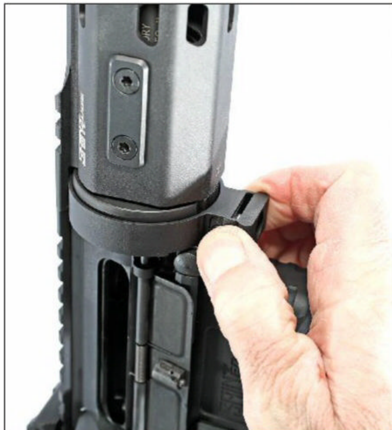
To take down the EVAC, lock the bolt back and then pull down the locking latch.
