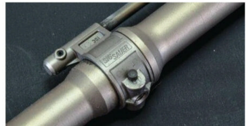
SIG's gas block is so fancy at first you might think it is adjustable, but it is not. It is pinned in place for the utmost in durability and reliability. That blowback and discoloration on the gas tube is normal after you've put hundreds of rounds through a gun.
