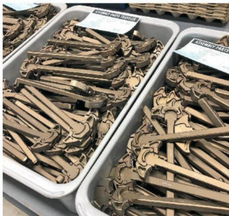
Two bins full of Airborne charging handles at the Geissele factory, done in their DDC anodizing, which stands for Desert Dirt Color.
