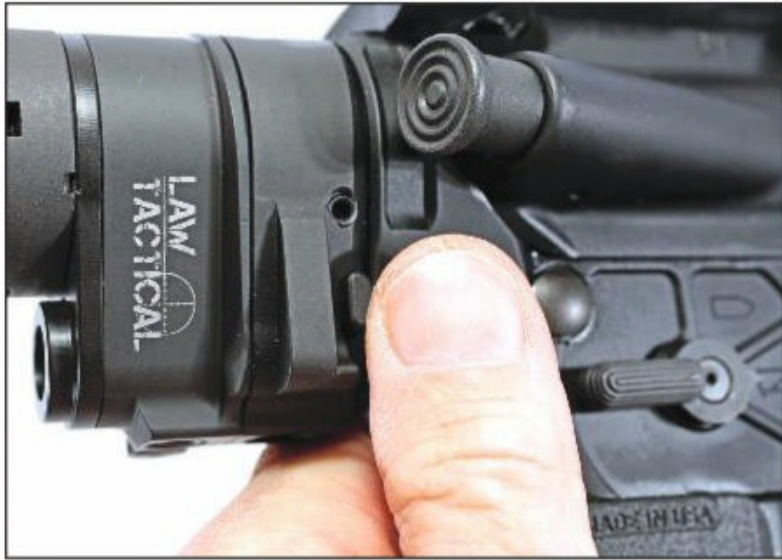
To fold the Law Tactical, you have to press the unlocking button.
