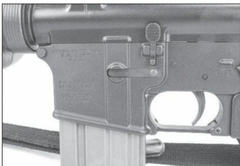
I actually built this M16A1 rifle up using a GhostGunner milling machine and a Hydramatic 80% lower receiver. The end result is a semiauto spitting image of the Vietnam-era M16A1 right down to the receiver markings.
