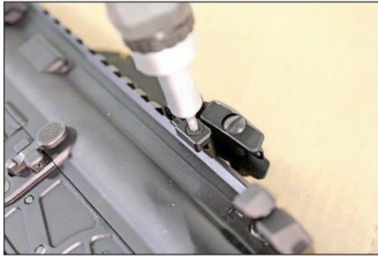
The Springfield sights are held onto the receiver by means of a torx screw. A T15 is the correct size, should you need to move the sights.
