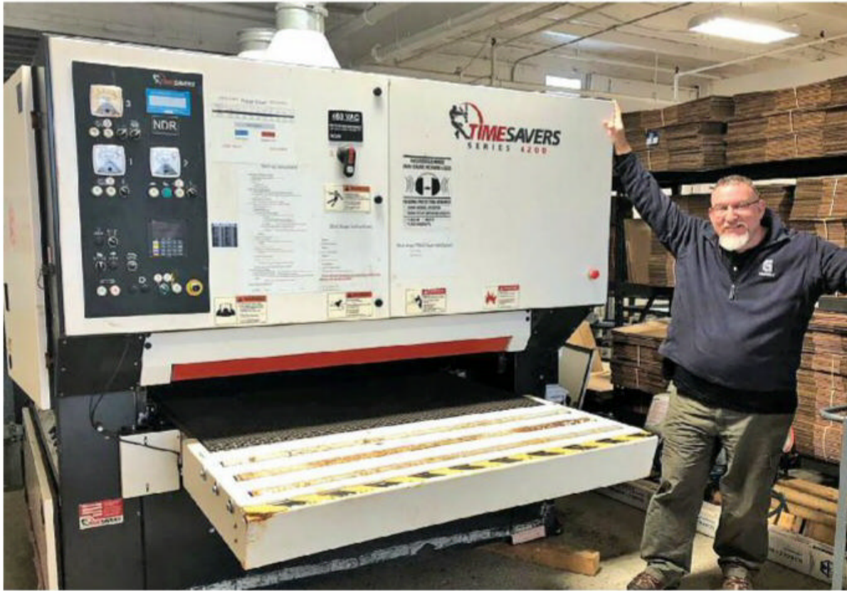
Bill Geissele standing in front of a machine bought through government surplus. This machine sands smooth the surface of steel plates that will become Abraham and Moses knives, a sister company run by his sons.
