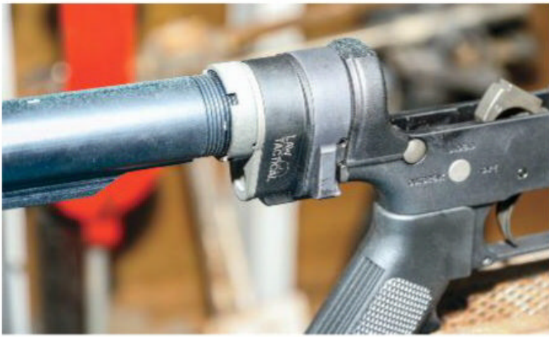
The sole job now of the lower retaining plate is to provide a location you can use to stake the castle nut, once you complete the build.
