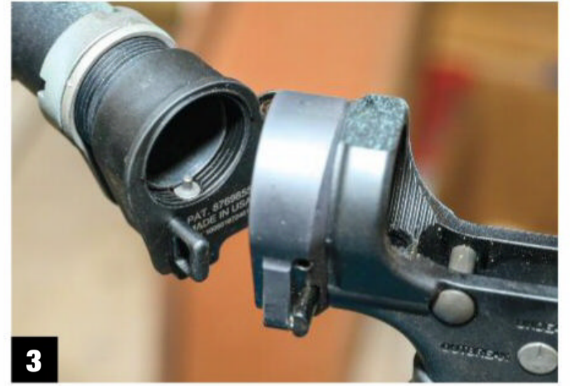
3 You install the buffer retainer in the adapter as you are also installing the buffer tube.
