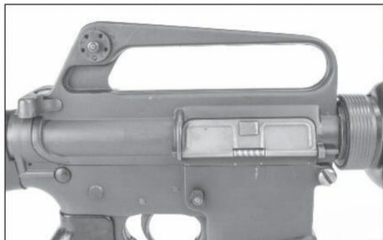
The earliest SP1 AR-15 rifles lacked a forward assist device, had their buffer tubes secured with a roll pin, and sported the little "plus" sign on the side of their lower receivers. The magazine catch was also left unprotected against accidental manipulation.
