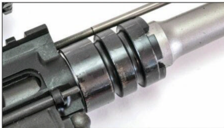
Swapping out one SIG handguard for another requires only removing two hex-head bolts which secure the handguard to this barrel nut. The barrel's light profile is apparent.
