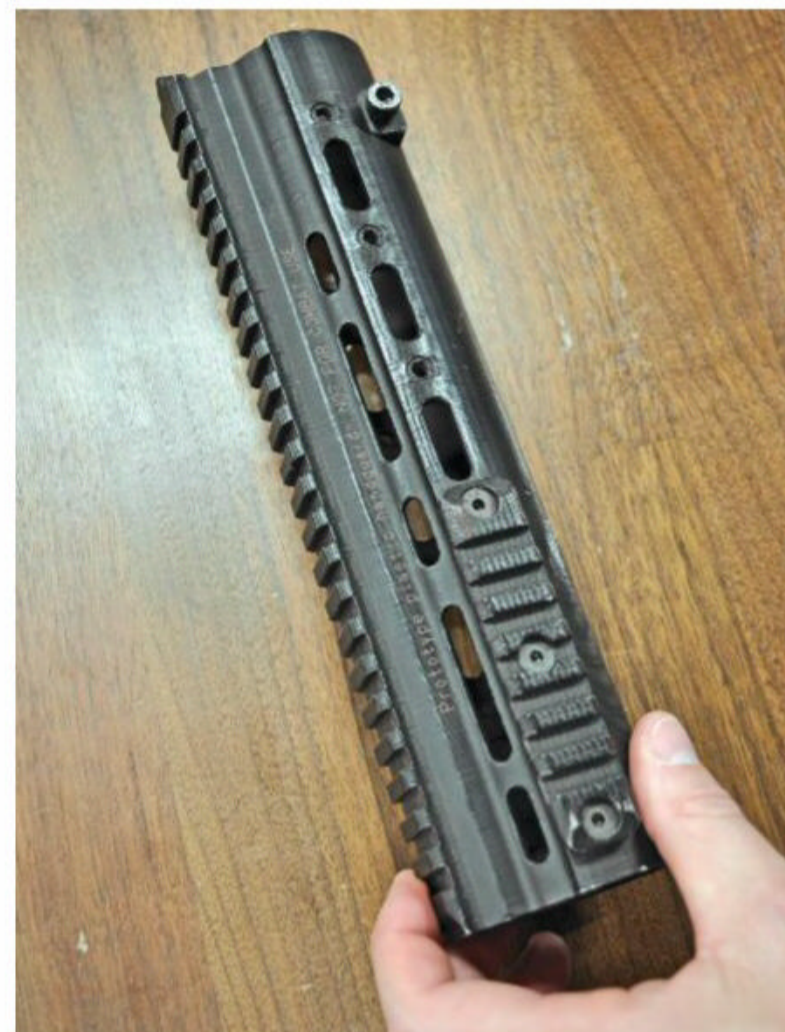
A 3D-printed prototype of Geissele's first rail design, for the HD 416. Note the "NOT FOR COMBAT USE" etched on it.
