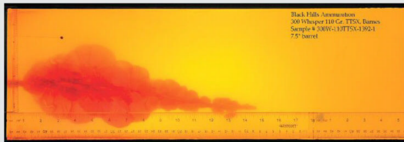
The Black Hills 110 grain TTSX load expands to over .600", penetrates to just over eighteen inches, and runs like a champ.
