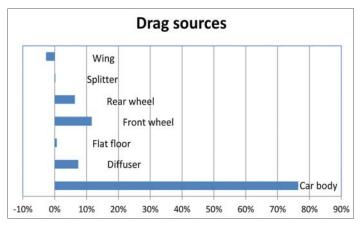
Figure 1: The sources of drag by major components; note the high number for car body
