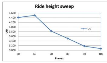
Figure 15: Ride height versus efficiency (-L/D). Drag reduced with each height reduction
