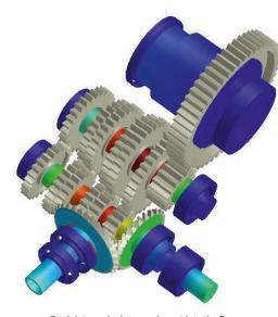
Real duty cycle data can be put into the Romax software which then helps Hewland determine exactly which bearing or gear mesh could be a limiting factor
