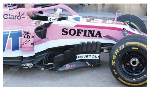
The area behind the front wheels is crucial for performance and its importance will grow in 2019 with the new aero regs
