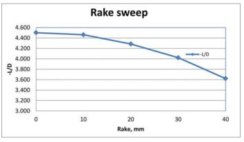
Figure 17: The rake at 60mm front ride height versus the aerodynamic efficiency (-L/D)
