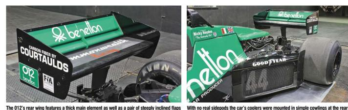
The 012's rear wing features a thick main element as well as a pair of steeply inclined flaps
