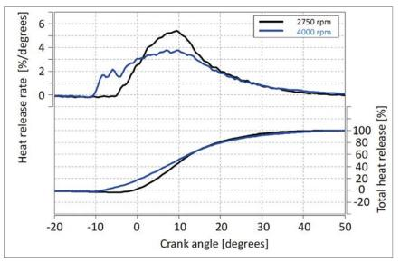
Figure 2: Heat release rate comparison between 2750rpm and 4000rpm. This shows optimum crank angle for maximum efficiency is 50 degrees which equates to 50 per cent mass fraction burned point of the combustion total energy per lap from the fuel and hybrid system combined. 2) Fuel tank capacity. 3) Maximum fuel flow rate.
