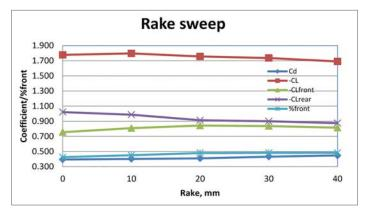
Figure 16: The rake at 60mm front ride height versus the car's aerodynamic coefficients
