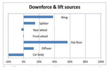
Figure 2: The sources of the downforce and lift; the car body also generated some lift
