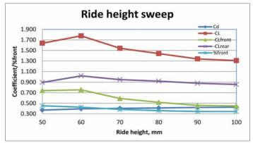
Figure 14: The effects of the ride height changes on the car's aerodynamic coefficients
