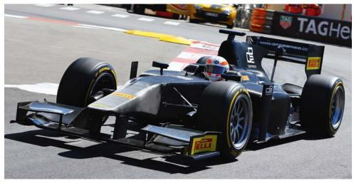
Pirelli tested 18in wheels fitted with low profile tyres on a GP2 car during a demonstration run at Monaco three years ago
