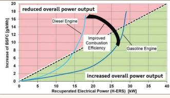
For a diesel engine the amount of electrical power that can be recuperated can lead to an increase in BSFC, resulting in increasing losses and overall lower power output be used to spin up the compressor resulting in immediate additional power with no turbo lag effect.
