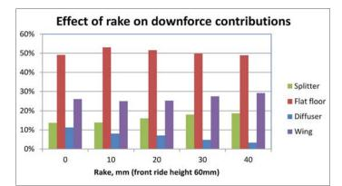
Figure 18: Contributions of main downforce producers with 60mm front ride height rake
