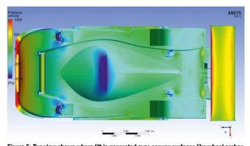
Figure 5: Top view shows where lift is generated over convex surfaces like wheel arches
