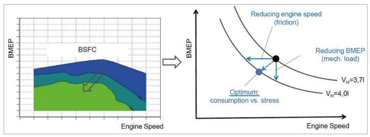
Figure 3: The increase in displacement from 3.7 to 4.0 was chosen on the basis that it not only improved fuel consumption for the same power but also reduced mechanical loads
