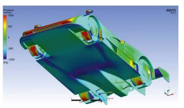
Figure 4: Pressure distributions on underside. Blue and green is decreased pressure
