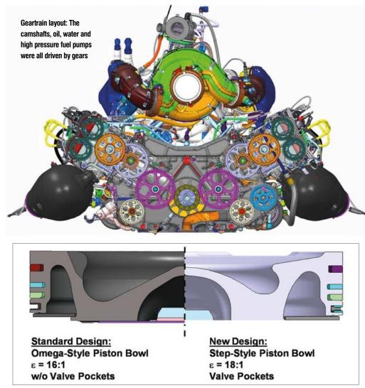
Cross section of the piston head showing development of piston bowl profile from the original (left) to new iteration (right)
