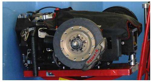
LMP brake discs have a larger diameter than those used in F1; it is possible the latter might use similar discs from 2021
