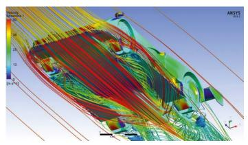
Figure 6: The streamlines show the 3D nature of the flows. Note the front wheel wakes
