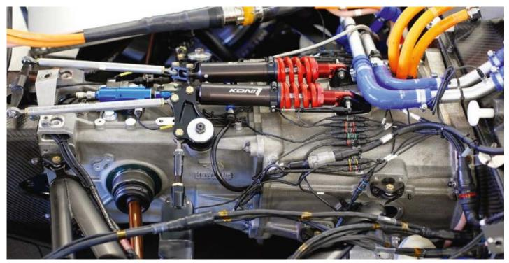
Hewland Formula E gearbox. Despite the slower speeds in FE designing a transmission to cope with the high regenerative loads from the electric motors has been a real challenge
