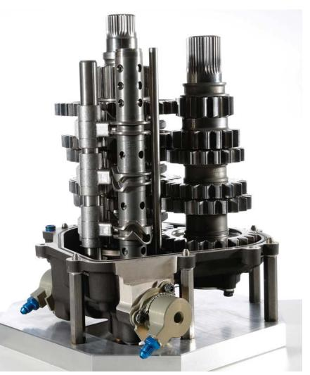
The gear cluster from Hewland's LMP2 transmission. The contact patches between the gear teeth need to be designed so the gears do not deflect or slide under load as this can generate heat, leading to inefficiencies
