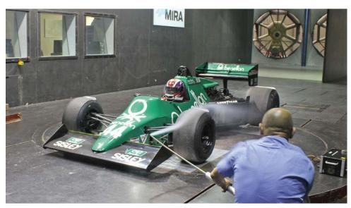
Tyrrell's 012 was the team's answer to the banning of ground effect sidepods for 1983. It featured a simple wing package, no sidepods and minimal floor area. Note the trip strips fitted to the wheels to better simulate the flows when wheels rotate
