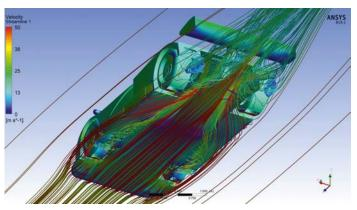
Figure 10: The inflow into the underbody along the car's sides is quite clear in this view
