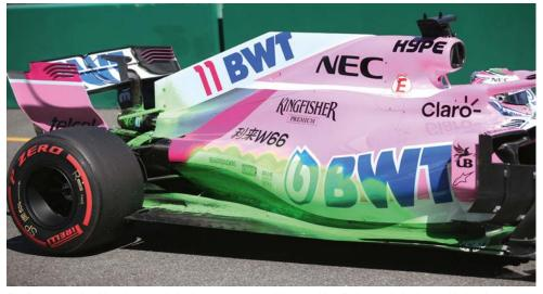
The flow around the sidepod was not behaving as expected and the team identified a correlation issue with the wind tunnel
