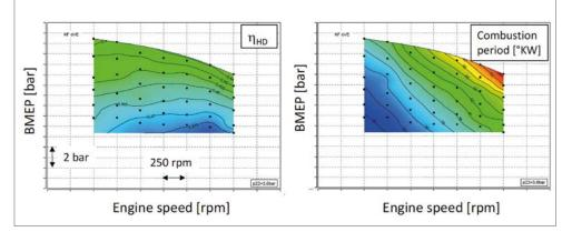
Figure 1: Typical map of 2013 unit. Left shows indicated combustion efficiency; right shows the period in the engine map
