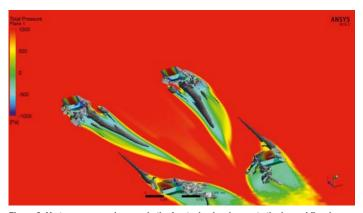
Figure 9: Vortex cores can be seen in the front wheel wakes; note the inward flow here
