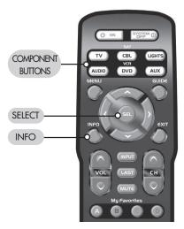
STEP 2: Press the INFO button and count the number of times the Component LED light blinks. This number indicates the first digit of the code. Next it will pause for about one second and begin blinking again to indicate the number of the second digit. Then once again it will pause, then blink, to indicate the number of the third digit.
