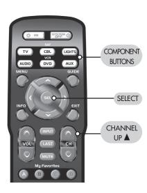
**STEP 3:** Press either the TV or CBL button that you want to use as the source of channel control. The component LED will blink three times to confirm it is saved.
