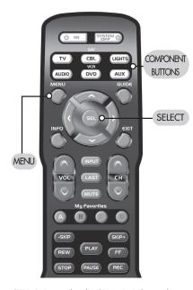
**STEP 3:** Press either the CBL or DVD button that you want to use as the source of OSD Control. The component LED will blink three times to confirm it is saved.
