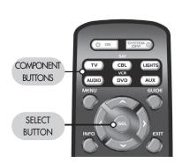
**STEP 5:** Point the URC-A6 toward the component (in this example the TV) and punch in the first 3-digit code that you wrote down for that specific component. Use the Number buttons 0–9 on the remote to punch in the code. The TV LED light will blink each time a number is pressed.
