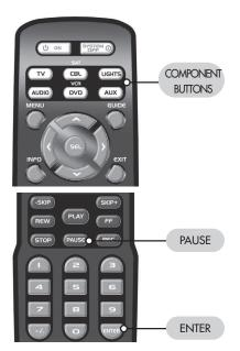
**STEP 3:** To exit Erase mode, press and hold both the component button and the ENTER (ENT) button at the same time until the component LED light blinks three times.
