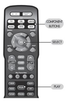
**STEP 3:** Press either the DVD or DVR button that you want to use as the source of Transport Control. The component LED will blink three times to confirm it is saved.
