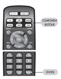
**STEP 2:** Press and hold the button you want to erase for two seconds. The component LED light will blink twice to confirm the erasure.
