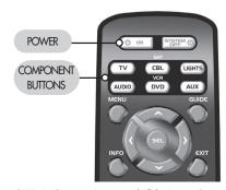
STEP 3: Once you've entered all the Power On commands, press the CHANNEL UP ▲ button to save your MacroPower commands. The component LED lights will blink three times to confirm that the programming has been successfully saved.
