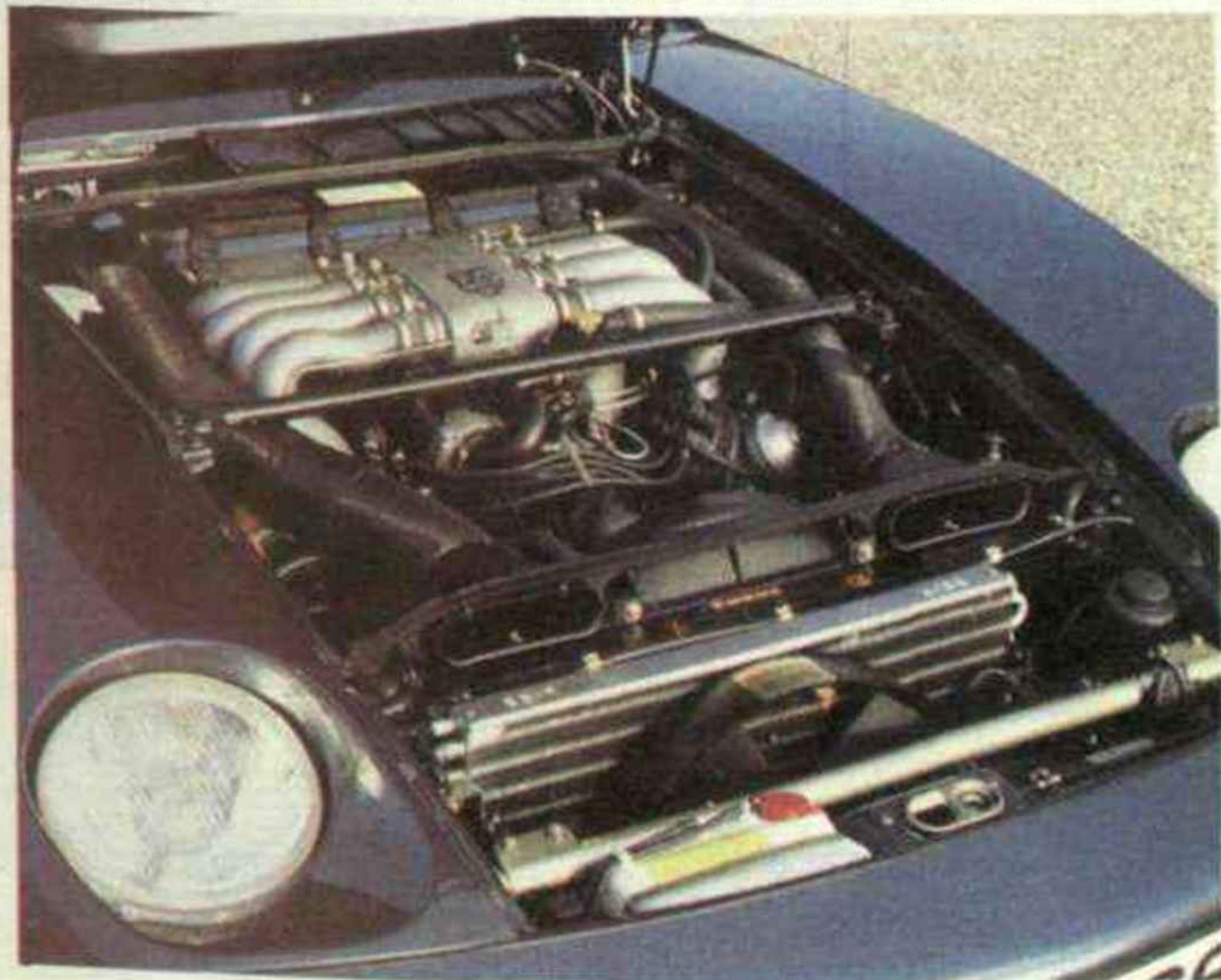
SYMMETRY IN ALUMINIUM. - The 240 b.h.p., 4.5-litre V8 sits right back behind the axle line. Oil is replenished through the filter bowl beneath the difficult to release yellow knob. This Porsche is nominally a four-seater.
