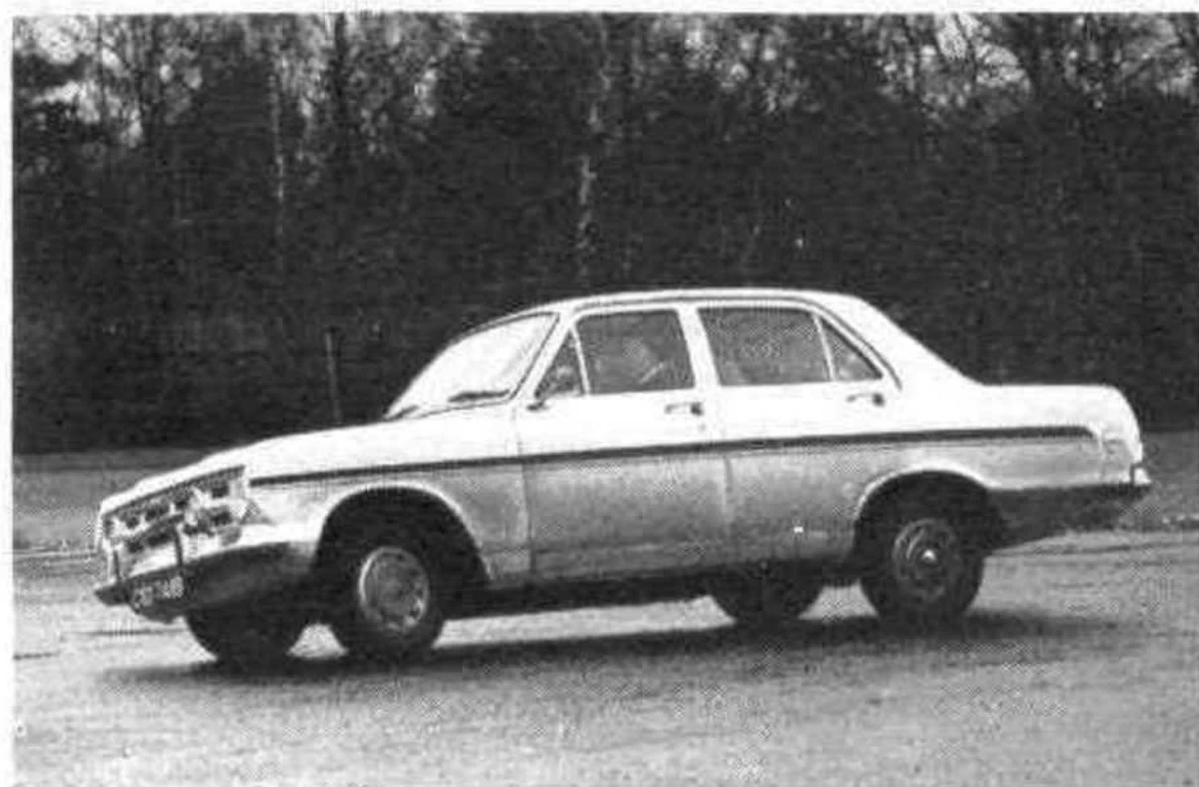
ROLLING. —The Vauxhall VX 4/90 objects to being cornered aggressively. It had a top speed of 96 m.p.h., covered a s.s. ¼-mile in 19.6 sec., and was a considerable improvement over the earlier versions.
