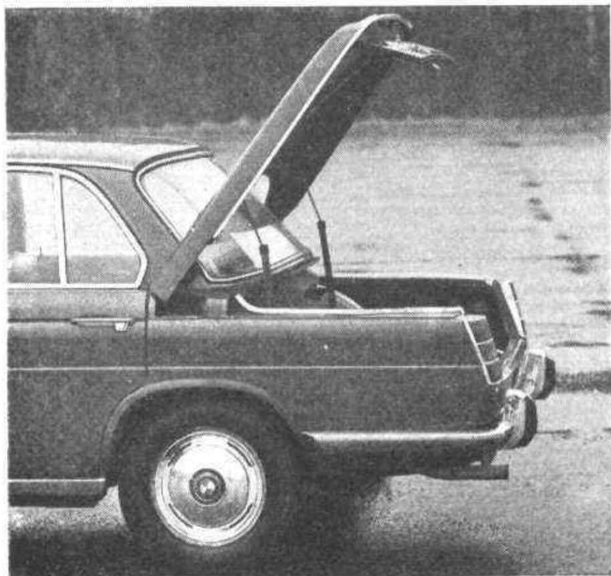
The B.M.W.'s boot has low-level loading by reason of the shape of the lid, which is retained in the open position by torsion bars.
