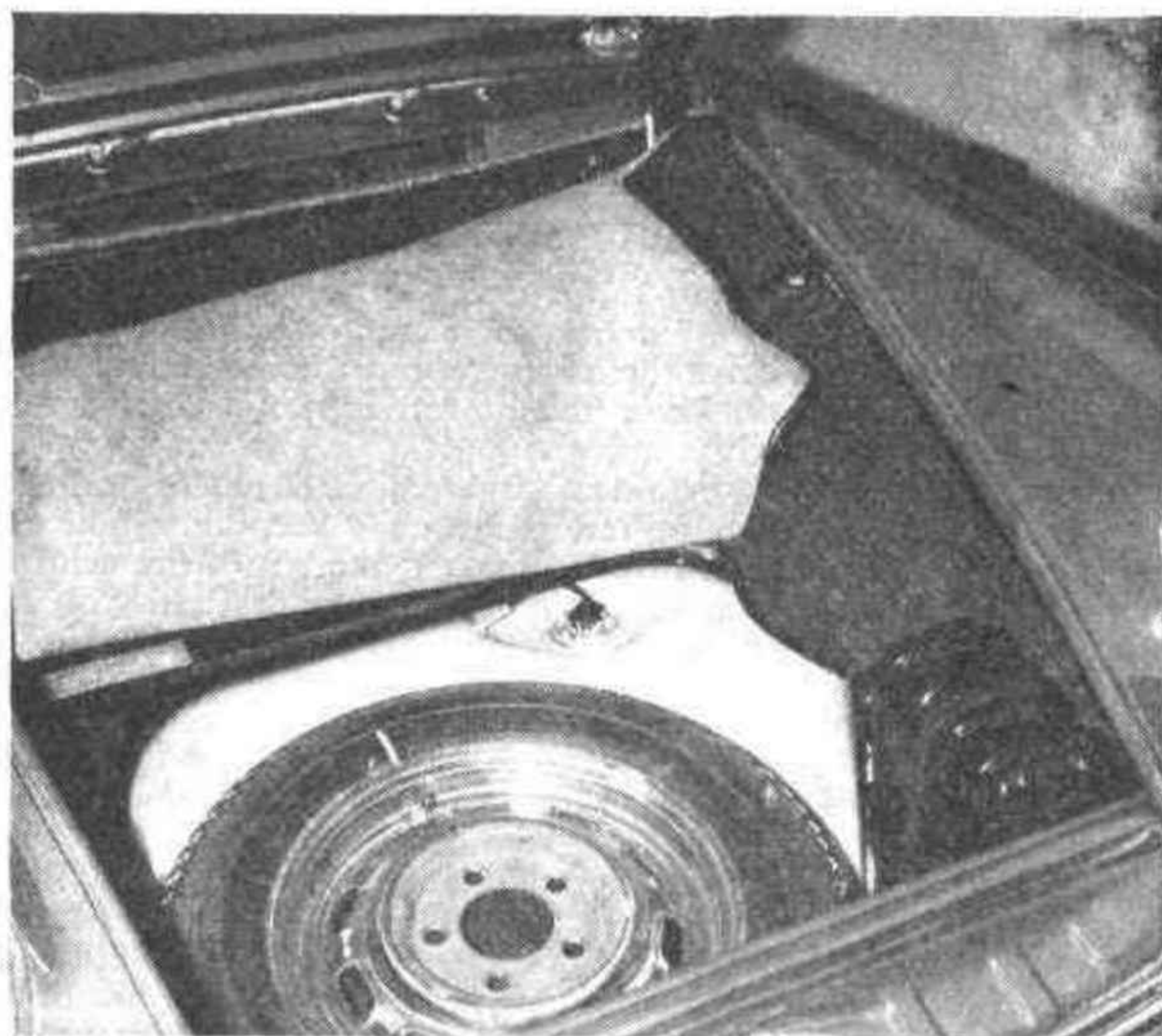
BONNET SPACE.—The spacious luggage compartment under the bonnet of the 911. The shaped fuel tank has the spare wheel fitted into it.
