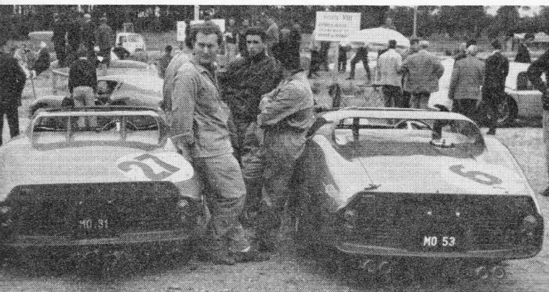
LEFT: The V8 Ferrari of Giancarlo Baghetti and Lodovico Scarfiotti (left) and the winning 4-litre V12 of Hill/Gendebien. Note the different exhaust systems and the strange aerodynamic "shelves" behind the drivers.
