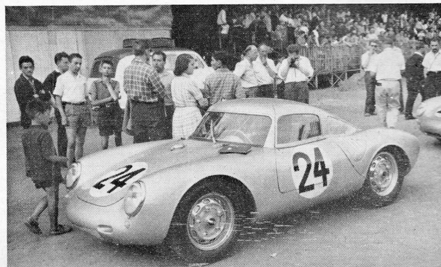
ULTRA-LOW were the works Porsche coupés, as demonstrated by a six year old French boy standing next to the Maglioli/Herrmann car. Access to the rear engine is provided solely by the side hatches, one per side, aft of the doors.
