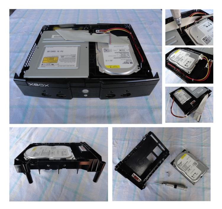
To remove the Hard Drive you will find the first Torx 10 screw underneath the IDE cable, next remove both the cable's attached to the Hard Drive. Untangle the power connector wire's from the Hard Drive mounting bracket, you can cut the cable ties to make this easier and lift up the whole thing. The Hard drive is held in the mounting bracket by four Torx 15 screws.
