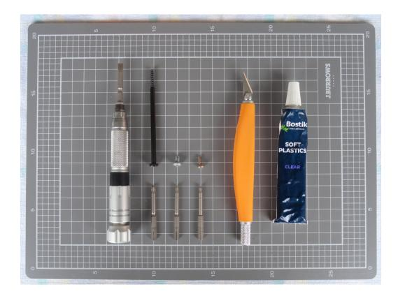
The main tool you will need to disassembly the Original Xbox is a Torx screwdriver set, in addition with a single flat-head screwdriver. My set in particular has interchangeable bits as shown in the image, above each Torx bit is there corresponding screws that they remove.
