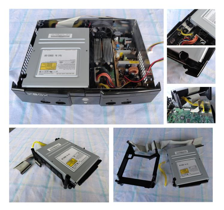
There are two Torx 10 screws on either side of the Disc Drive (DVD-rom) towards the front of the console just behind the faceplate. Lift the Disc Drive and mounting bracket then unplug the two cable's from the motherboard. From here you can remove the cables from the Disc Drive and pop it out from the mounting bracket which is only held in by a couple of clips towards the back of the Disc Drive.
