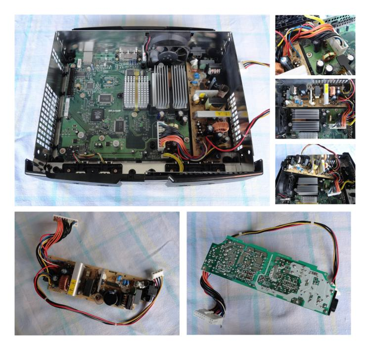
Unplugging the dual row PSU connector is fairly straight forward but single row PSU connector found on v1.0 and v1.1 consoles can be a bit more difficult, just pay attention. There will be two Torx 10 screws along the edge of the Power Supply Unit closest to the Motherboard. Once both screws have been removed slide the PSU towards the front of the console and lift it from the back while being careful not to break the plastic tabs along the right hand side of the case.
