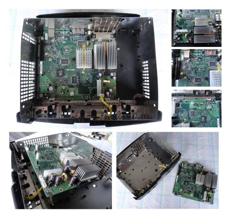
With all the other components removed all that remains is the Motherboard. Depending on your console version there will be either ten or eleven Torx 10 screws on the Motherboard that need to be removed, lift the Motherboard from the front to about a 45 degree angle and gently pull it out. Sometimes the shielding around the Ethernet and Video/Audio connector can be rather tight, just keep wiggling the Motherboard until it finally breaks free.
