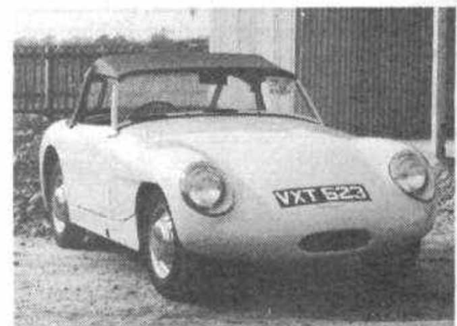
WHAT became known as the 'Costin nose' first appeared on the Speedwell Sprite.
