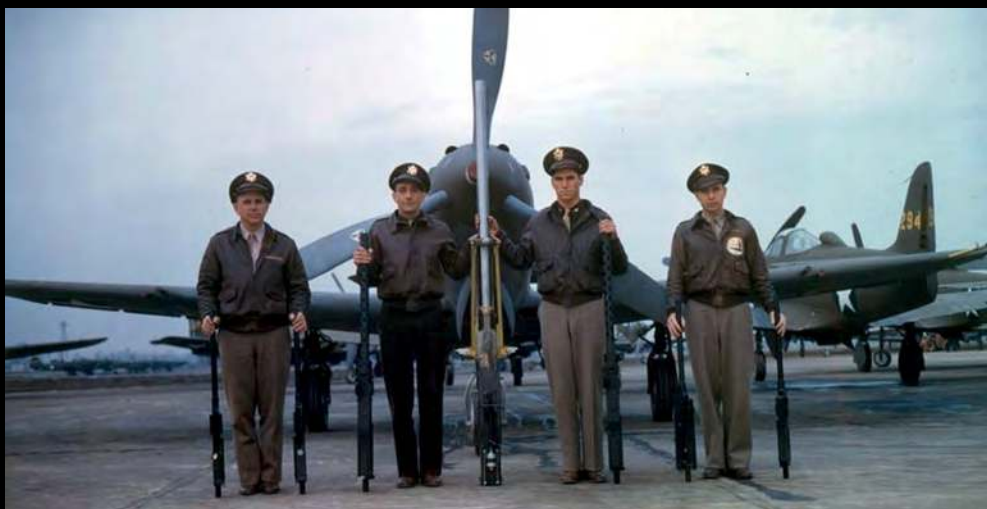
Below With guns blazing, this iconic photo of the P-39 graphically shows its impressive armament of four .30-cal and two .50-cal machine guns, and one 37mm cannon. USAF
