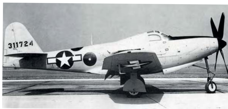
Left Flying target: Operation Pinball involved Kingcobras being flown for gunnery training as the recipients of 'live' firing with frangible bullets. Shown here is 43-11724, an RP-63G-1-BE, which was the final version intended for the Pinball programme.
