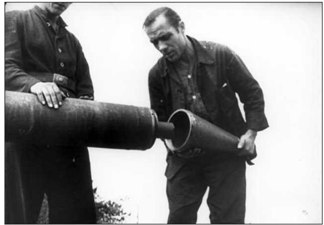
mando Tröller and civilian engineers from Rheinmetall-Borsig. (IWM) Right: The warhead was already attached to the fourth stage when this was fitted (see picture left), which might suggest that it was not live. Here technicians mount the nose cone of the rocket on top of the percussion fuse. (IWM)
