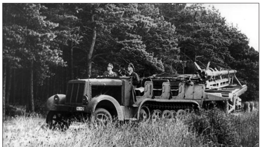
Powerful half-track prime-movers were needed to manoeuvre the heavy Meiller trailers (nearly 12 tonnes when a rocket was transported). Here, an FR-Wagen is being towed into position by an SdKfz 7 half-track at Waldheim during the operational training of Artillerie-Abteilung 709.
