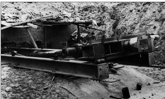
Left: The gun was under repair when the picture was taken. The breech had been unscrewed from the barrel (off the picture to the right) and turned upside down, consequently, the rear of the breech is facing the barrel (see also page 3, top left). (Bundesarchiv) Right: The Hillersleben test range lies north of the
