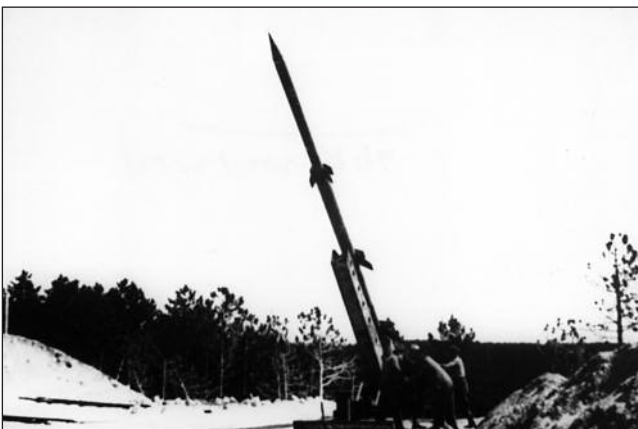
Left: With the rocket ready for the launch, the ramp was raised by hand-cranking it up to the proper elevation of 64 degrees which had been calculated as giving the maximum practical range. (IWM) Right: From the shelter of a dune some distance away, the cameraman filmed the launch of the rocket which
