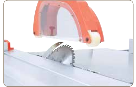
Saw unit – tiltable up to 45° - can be adjusted by handwheel for cutting heights up to 90 mm.
