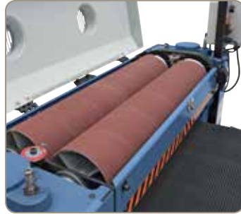
2 sanding rollers for rough and fine grinding in one pass.
