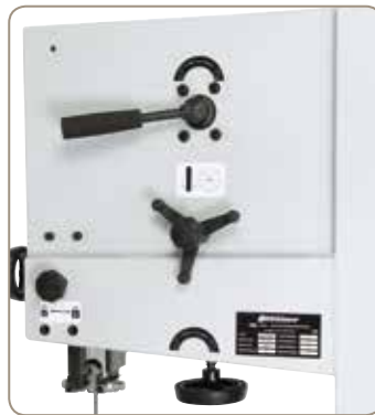
Easy bandsaw blade changing using a quick clamping lever, the basic setting of the drive wheel will not be changed.
