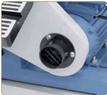
Serially with 2 dust extraction outlets diam. 50 mm.
