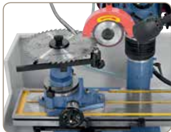
Sharpening of sawblade.
