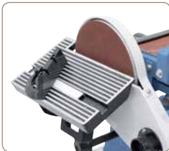
Sanding table tilts from 0° to 45°.
