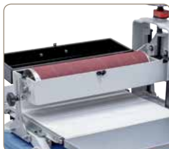
Lift dust hood to change the sanding belt.
