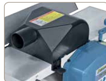
Combined dust hood can be used for surface planing or thicknessing.
