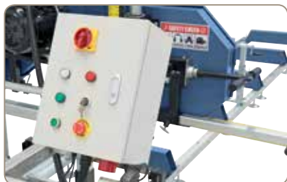
Picture shows electronic panel and push stick for manual feed (height adjustable).
