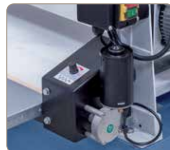
Variable feed adjustment.
