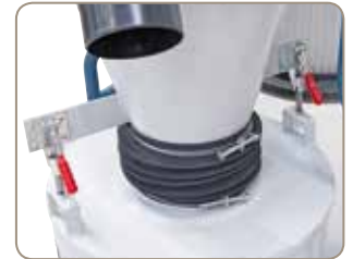
Serially with quick clamping lever for an easy access to the collecting vessel
