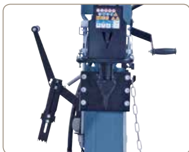
Two-handed safety operation for safe work, forward speed alternatively fast or slow.
