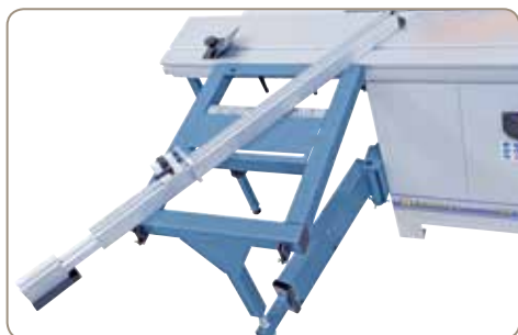
Steplessly tiltable telescopic arm (2 x 45°) can be mounted at front or rear of square table.
