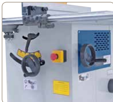
Ergonomic mounted handwheels allow for height adjustment and tilting of the saw unit.
