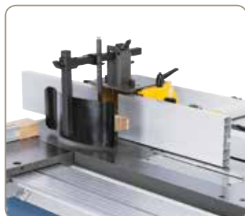
Solid moulding fence can be used for tools with a diameter of up to 140 mm.
