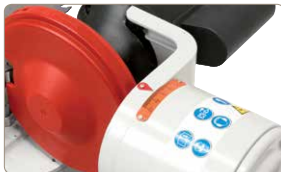
Tilts 33° to right and 20° to left, ideal for sharpening of ATB (alternate top bevel) sawblades.
