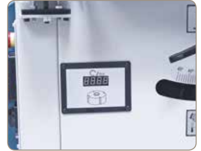
Electronic display of spindle speed settings.
