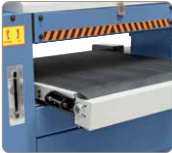
Adjustment screw for parallel run of the conveyor belt.
