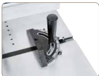
Mitre fence moveable along entire table length.
