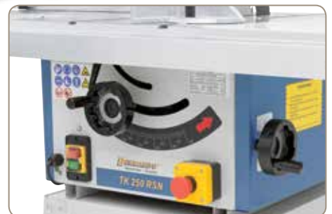
Ergonomically arranged handwheels on machine body allow for adjustment of saw unit.
