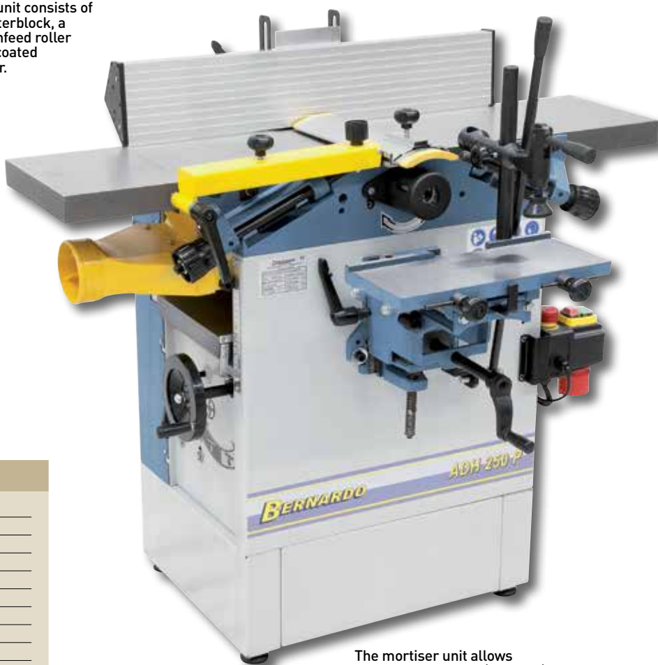
The planing tables are designed with slots to keep noise levels to a minimum.
