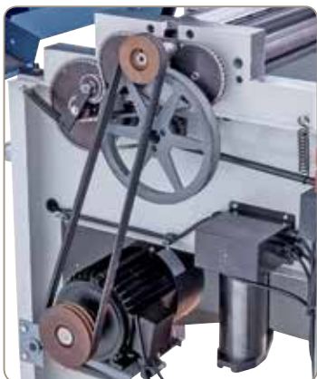
The chain drive ensures consistency of infeed and outfeed rollers.
