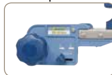
Scale for setting the edge protrusion
