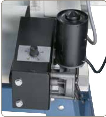
Variable feed adjustment.
