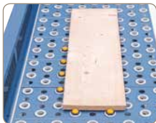
Standard with stops for positioning the workpiece.
