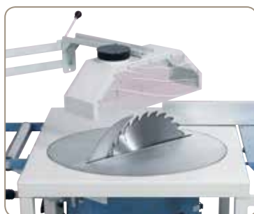
The protective cover follows the sawblade movement.
