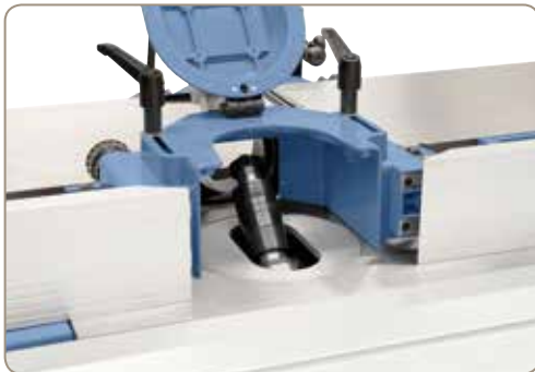
Milling spindle tilts to the back, bringing several advantages, such as optimal use of the power feed, maximum safety and tidy milling results.
