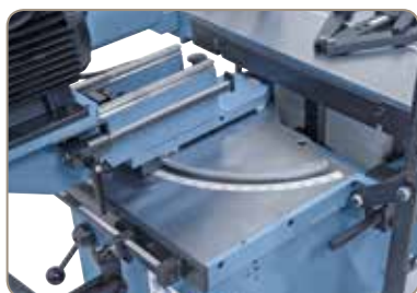
Drill head tilts 60° to right and left.
