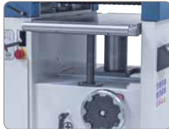
Solid thickening table with spindle guide and support for accurate planing of board, slats, planks etc.
