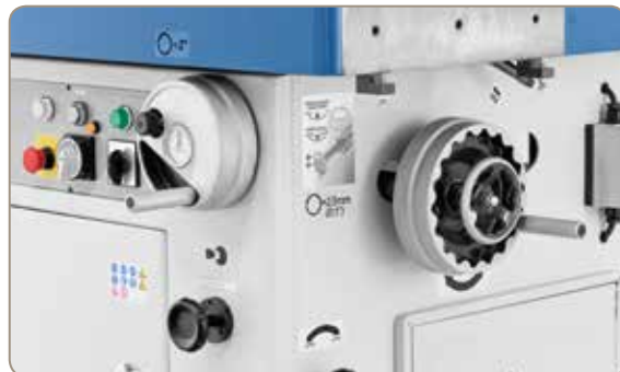
Oversize handwheels allow for precise adjustment of milling spindle.
