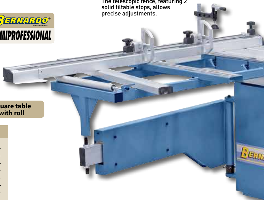
When cutting large pieces, parallel fence can be tilted down.
