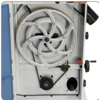
The desired cutting speed is adjustable with a V-belt at the lower flywheel (HBS 400 N / HBS 460 N).
