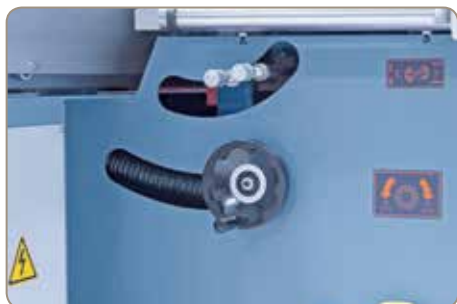
User-friendly height and side adjustment of scoring unit.
