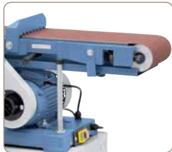
Large face sanding area with workpiece fence.
