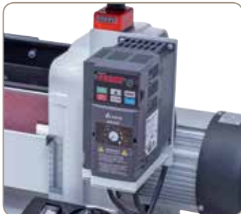
High-quality frequency converter allows for stepless adjustment of the spindle speed.
