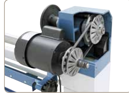
The solid variator-drive guarantees ideal power transmission
