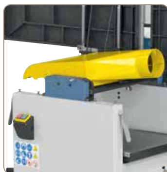
Integrated, tiltable dust hood – extraction outlet 120 mm.
