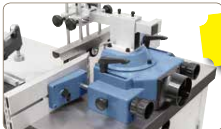
The solid moulding fence can be adjusted for tools up to 200 mm. Stop bars on both sides feature fine adjustment.
