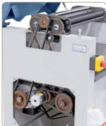
The infeed is driven by a solid chain drive. The infeed speed is 5 - 7 m/min.
