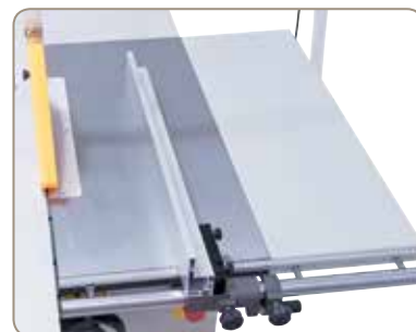
Parallel fence with quick and fine adjustment for cutting width up to 620 mm.
