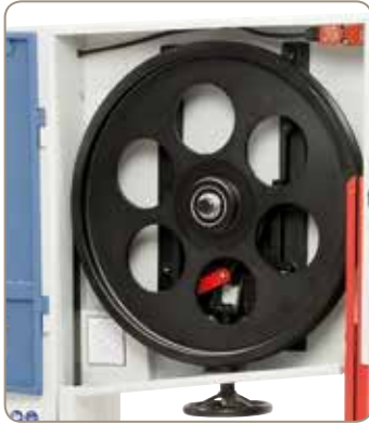
Dynamically balanced cast iron flywheels for smooth run.
