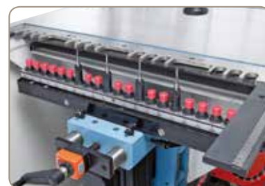
Fence with 3 gaps to use with multiple drill heads for hinges
