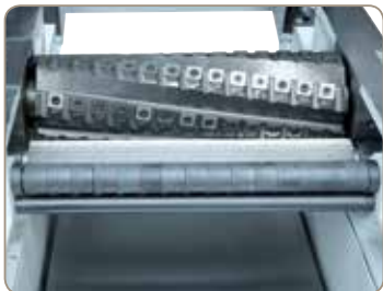
The precisely bedded spiral cutter head and the straight toothed of the infeed roller ensure top work results.
