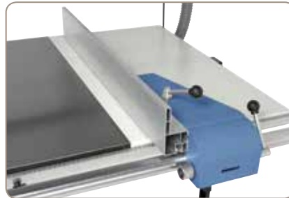
Tiltable parallel fence with micro-metric fine adjustment (advantage with oversize panels).
