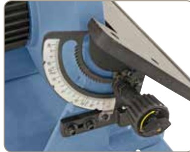
Polished grey cast-iron table with tilting range from -3° to +45°
