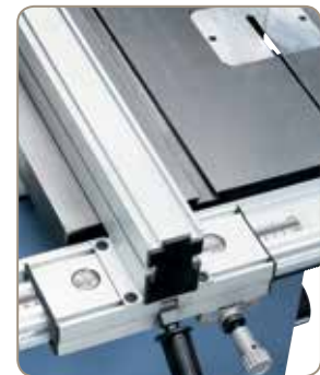
The integrated loupe at the rip fence afford an exact read-off of the adjusted cutting width, HBS 500 N additional with fine adjustment.
