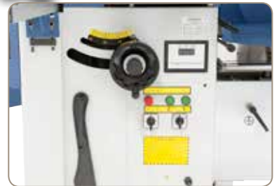
Electronic display of spindle speed settings.
