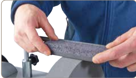
05-2050 Stone grader: Suitable for thorough preparation of grinding wheel (fine / rough).
