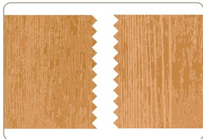
Prong bonding of boards guarantees high rigidity and maximum strength
