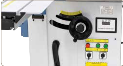
Electronic display of spindle speed settings.
