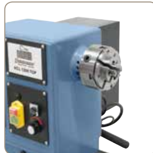
Power chuck set Premium M 115, Stepped jaws
