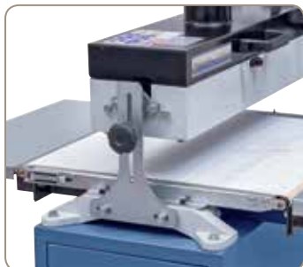
Clamping system allows fixing the grinding unit into position.
