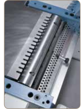
The table lips in combination with the perforated chip plate keep the noise level to a minimum.
