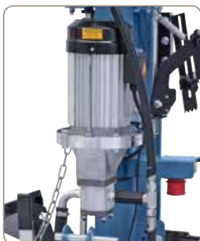
ZE-models with powerful electro motor and high quality hydraulic pump.
