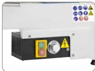
Stepless adjustment ensures ideal speed settings.
