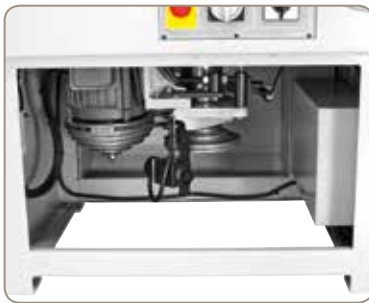
Oversize opening on machine front allows for easy belt change to adjust speed.
