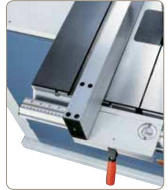
Easy adjustable aluminium rip fence with quick clamping system, read off the mm-scale by loupe.
