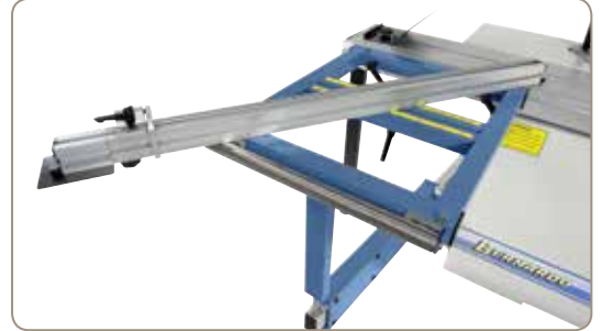
The steplessly tiltable telescopic fence (2x 45°) can be mounted at the front or rear of the square table.
