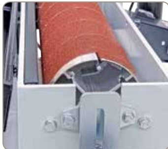
Quick clamp system for sanding belt.
