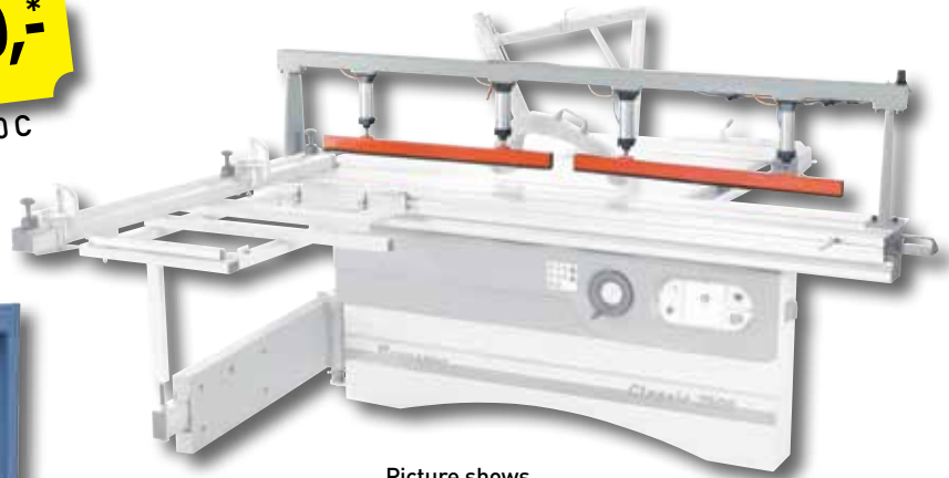
Picture shows optionally available pneumatic clamping device.
