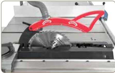
Complete with scoring unit for burr-free processing of sheet materials.
