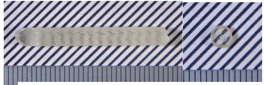
0.25-1mol% Pr-doped \text{Lu}_3(\text{Al,Ga})_5\text{O}_{12} micropulling-down grown, IMRAM, Tohoku university, Sendai, Japan
