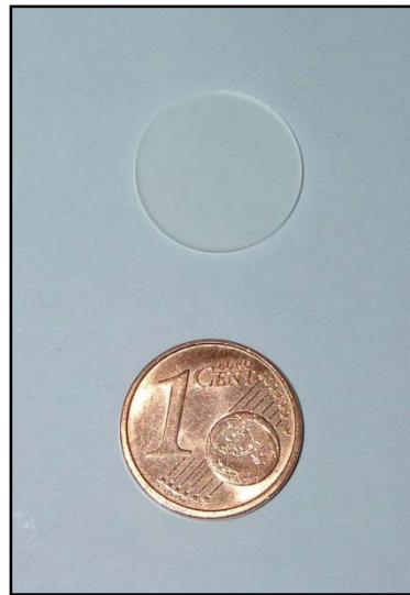
Ce-doped silica glass, DMS-University of Milano-Bicocca
