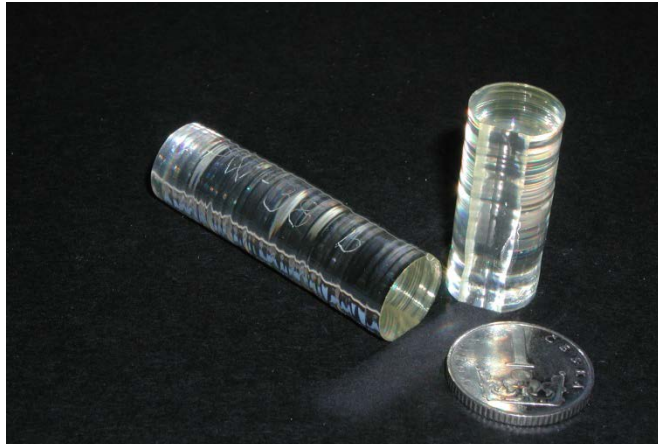
Czochralski grown \text{PbWO}_4 , IP Prague
