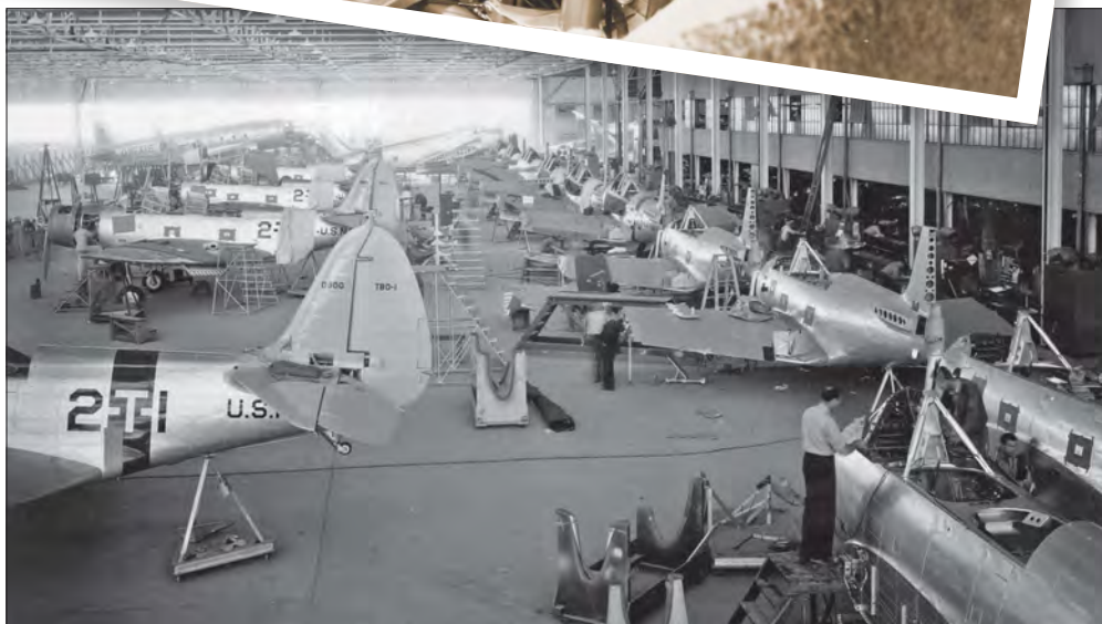
Right: Douglas TBD-1 torpedo bombers pictured in various stages of assembly at Douglas Aircraft Company's Santa Monica, CA, plant. Note that the aircraft already carry the markings of Torpedo Squadron 2 (VT-2), which received its first delivery of Devastators in 1938.
