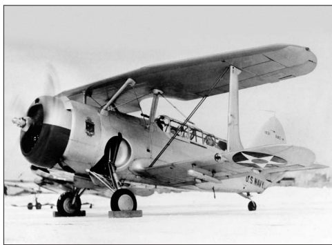
Above: A chilly scene at Naval Air Reserve Air Base Minneapolis as Curtiss SBC-4 Helldiver (BuNo 1831) starts up. Reserve Scouting Squadron Ten (VS-10R) and Marine Reserve Scouting Squadron Six (VMS-6R) operated SBC-4s at the base. Note the Naval Air Reserve insignia on the aircraft's cowling.
