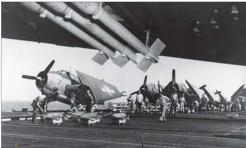
Below: Ordnancemen on the flight deck of an unidentified escort carrier, prepare 12.7cm High Velocity Aircraft Rockets (HVAR) and 227kg bombs for loading onto Grumman TBM-3s. The rockets allowed Avenger crews to strike at surface targets with devastating results to the enemy, both physically and psychologically.
