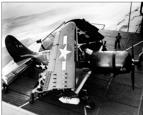
Above: Plane handlers manoeuvre SB2C-5 of VB-95 into the hangar deck of USS Bunker Hill (CV-17) during operations in the Pacific. Note that the Helldiver only just fits on the elevator, one of the reasons why its fuselage could not be extended to improve its handling.
