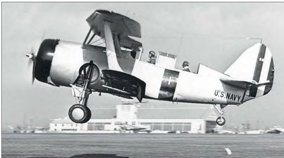
Left: A US Navy Helldiver making a simulated carrier approach during land-based training in preparation for operations at sea. The Helldiver design was characterised by its staggered, uneven span biplane wing arrangement with thick outboard struts, cabling and skeletal inboard struts designed to hold the wings in place during dive-bombing operations.
