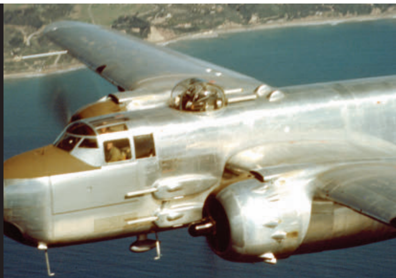
Not all aircraft in service had external deflectors as shown on this B-25H behind the top turret. Their function was to protect the tailgunner, when the top turret guns were stowed facing aft, in the event a round "cooked off" due to the guns being hot.
