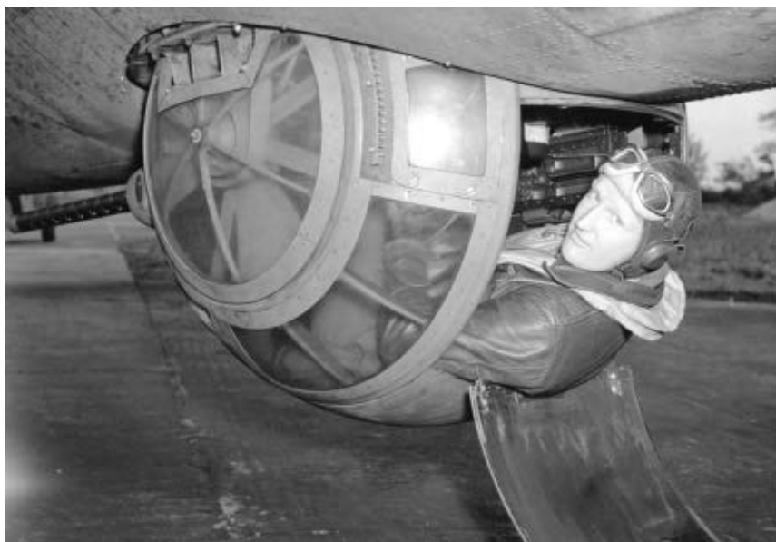
Top: Introduced on the B-17E, the Sperry top and belly power turrets with computing sights provided an effective defense against high-speed Luftwaffe fighter attacks. (Photo courtesy of Stan Piet)
