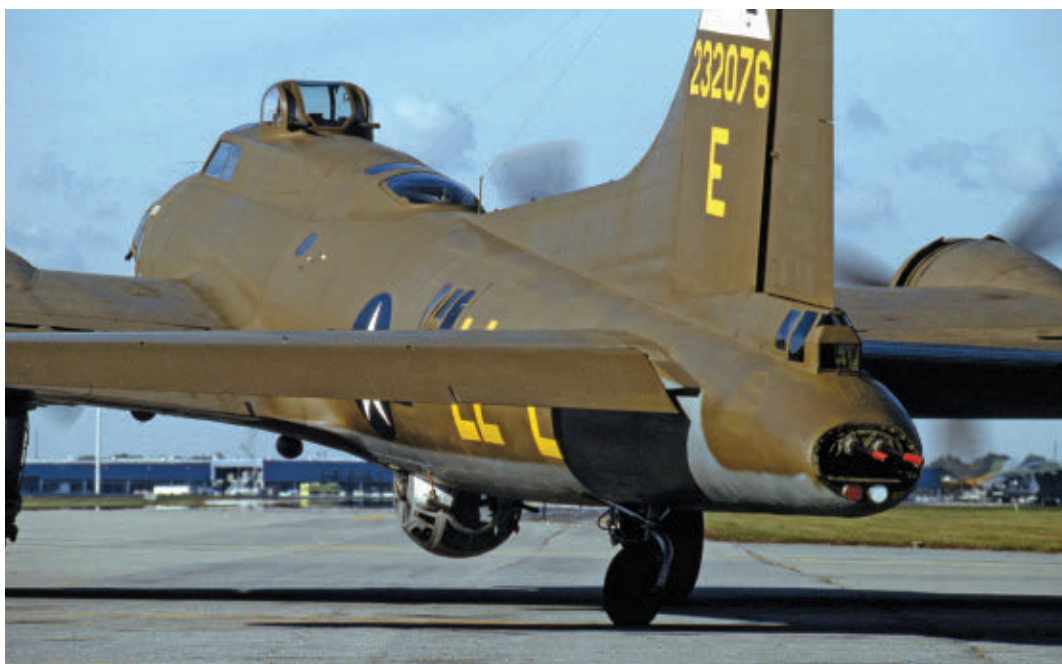
From this vantage point, it's obvious that this was a very dangerous position for a fighter because, including the dorsal gun, a total of seven fifty-caliber Brownings could be trained on it. As soon as the fighter was directly astern, only the two tail guns could be brought to bear. (Photo by Budd Davisson)
