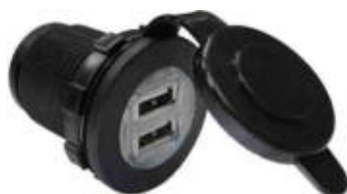
W4 compact double USB socket 12/24V with reverse polarity protection. LED power indicator. 36.8mm ø. 40mm depth. Output : 5V DC 2.1A Max. No data transmission possible 010648
