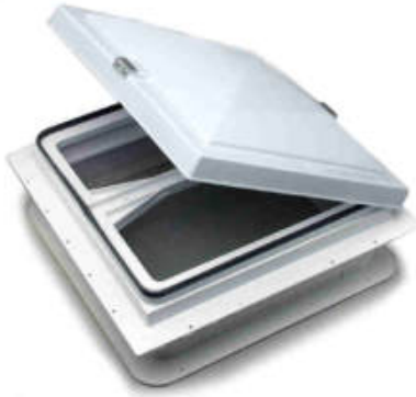
Elixir rooflight Single glazed unit with one way wind up mechanism. Metal surround. To fit aperture size: 360mm x 360mm White 102033 Spare dome only White 102037
