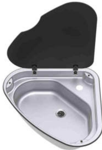
Basic Line 33 25mm waste outlet, plug, seal, 35mm tap hole and lid included. Dimensions: Cut out: 460 x 460mm. Overall: H140 x W480 x D480 mm Inside bowl: H92 x W455 x D276mm Left hand 091155B Right hand 091155A as shown
