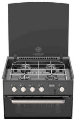
Minigrill 4 Burner Hob & Grill 4 burner 5.5kW (3 x 1.5kW and 1 x 1kW) hob with 1.6kW 13L grill. Comes with grill pan. 12V ignition. Dimensions: H x W x D mm Overall: 311 x 513 x 500 Build in: 312 x 496 x 490 091172C
