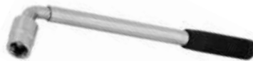
Master wheel wrench Chrome plated carbon steel body with 17/19mm vanadium socket. Telescopic handle gives adjustable length. 350-530mm. Product supplier changes occasionally Singly or 10 per outer 007169A
