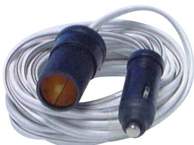
W4 cigar plug/socket lead Adaptor lead to extend lighter type sockets to a distance of 2 or 5 metres. Fuse (5 amp) built into plug. Singly or 10 per outer 2m 011675 5m 011680
