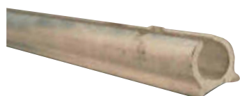
Aluminium awning rail 4mm opening. 9mm internal diameter, 12mm external. 10 lengths per outer 1.55 metre lengths 105099A 2.12 metre lengths 105099 2.7 metre lengths 105099B
