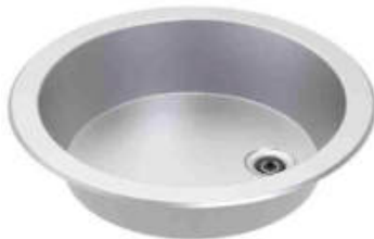
Series 23 spun bowl 25mm waste outlet, plug, seal and lid included. Dimensions: Cut out: Ø405mm. Overall: Ø460 x D123mm Inside bowl: Ø397 x D123mm 091158B
