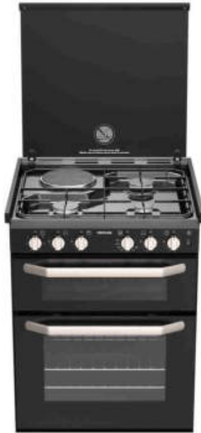
K1520 Dual Fuel 3 Burner Gas, 1 Hotplate Hob, Fan Assisted Oven & Grill 3 burner 4.2kW (2 x 1.6kW and 1 x 1kW) gas, and a 1kW electric hotplate hob with 2kW 37L oven and 1.8kW 19L grill. Comes with grill pan and 2 shelves. 12V ignition. Dimensions: H x W x D mm Overall: 645 x 515 x 501 Build in: 646 x 496 x 493 091188A
