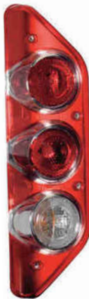
Caraluna modular Dimensions (HxWxD): 612 x 163 x 92mm Left hand 014490
