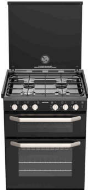
K1520 4 Burner Gas Hob, Fan Assisted Oven & Grill 4 burner 5.8kW (3 x 1.6kW and 1 x 1kW) gas hob with 2kW 37L oven and 1.8kW 19L grill. Comes with grill pan and 2 shelves. 12V ignition. Dimensions: H x W x D mm Overall: 645 x 515 x 501 Build in: 646 x 496 x 493 091187C
