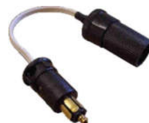
W4 adapt-it 5 Single pole plug to lighter type socket adaptor. 8 amp. Hella type. Singly or 5 per outer 011657
