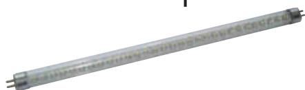
LED tubes Includes instructions on how to replace 8W fluorescent tubes with an LED tube. Under no circumstances should the tube be simply swapped. It must be wired directly to the 12V DC supply. T5 LED30 tube 018044
