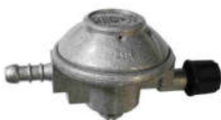
Gaz regulator For use with Campingaz cylinders. Integral control valve. Outlet pressure 29mbar 0.8Kg/h. EN 12864 approved. Singly or 10 per outer 070342
