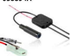
Active Splitter AS2611 Amplifies the signal from the aerial and provides FM and DAB+ inputs for the radio, with +20dB gain. For use with passive aerials (038895D) 038895A
