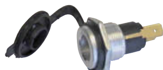
W4 DIN socket Single pole 12V, 19A flush fitting socket. For flush fitting in a 18mm Ø hole. 011631
