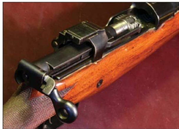
The Ross's interrupted-thread locking lugs were modeled on naval guns of the time, and were immensely strong – reputedly able to withstand 120,000 psi. Charles Newton copied the lug design for his rifles, and the later Weatherby Mark V was a variation on it.
