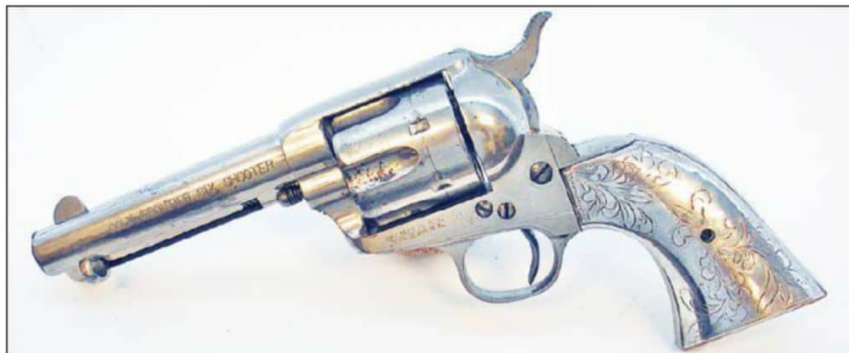
Colt Single Action Army .44-caliber barrels have remained .427 inch from the introduction of the .44 WCF in 1878.
