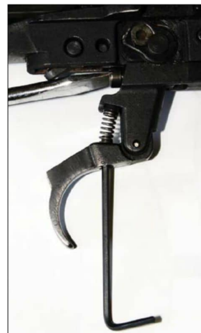
Original Ruger M77 bolt-action rifles include a user-adjustable trigger. Tweaking the trigger requires removing the action from the stock, a small flat-head screwdriver and tiny Allen wrench.
