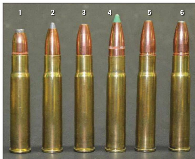
The .375 JDJ chamber throat is long enough to seat bullets with their bases no deeper in the case than the shoulder/neck junction: (1) Sierra 200-grain FN, (2) Sierra 250-grain SBT, (3) Swift 250-grain A-Frame, (4) Nosler 260-grain Ballistic Tip, (5) Swift 270-grain A-Frame, (6) Swift 270-grain A-frame.
