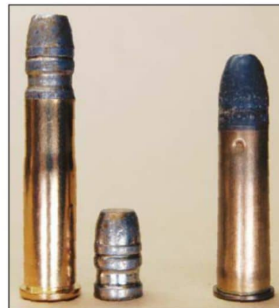
A new, unfired Starline .32-20 case would fit in the .310 chamber once the rim was thinned. The case was loaded with a pistol bullet. The bullet still didn’t touch the throat (left). A factory .310 cartridge is shown at right.
