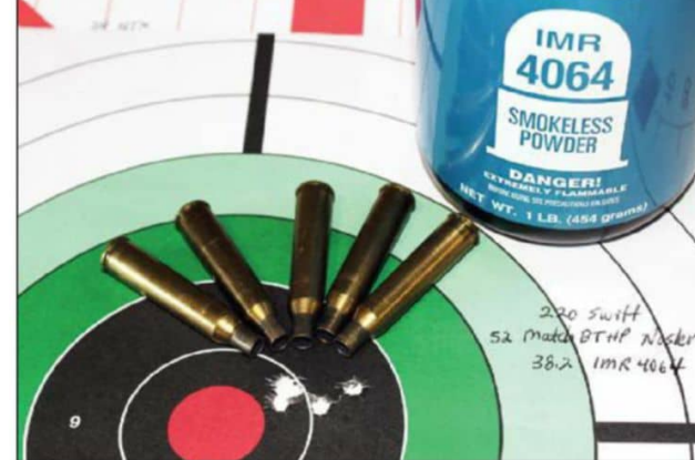
This handload of 38.2 grains of IMR-4064 beneath a Nosler 52-grain Match BTHP bullet proved to be the most accurate load tested.
