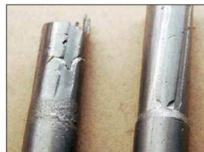
A chamber cast of a .310 throat (left) shows it to be just a tapered hole. A .30-30 is shown at right for comparison.
