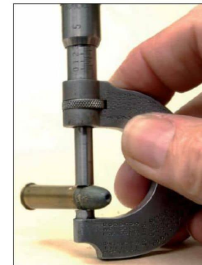
A micrometer shows the diameter of an unhandled .310 bullet is .327/.328 inch, but this is over dried lube.
