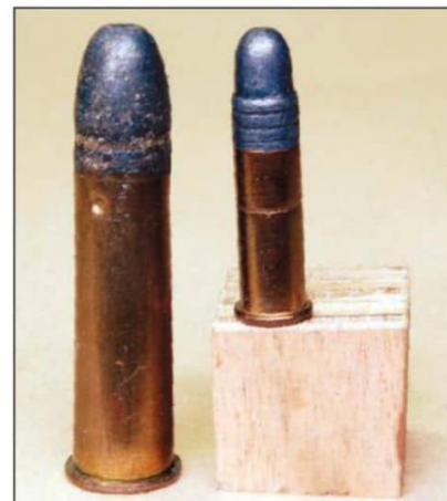
The .310 Cadet used an outside lubed bullet (left) just like the .22 rimfire (right).
