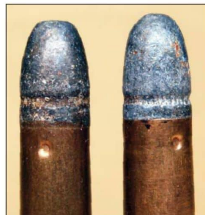
A Kynoch “stab crimp” of three indentations spaced 120 degrees around the case neck.
