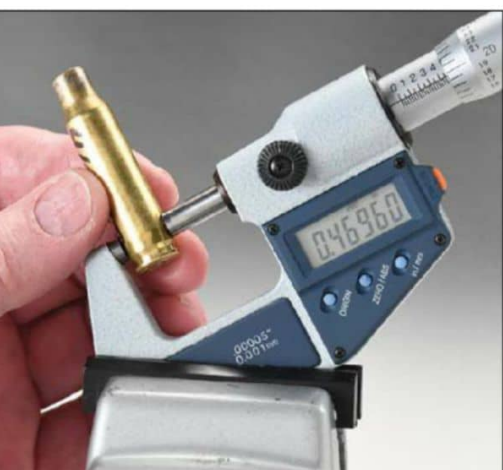
If measuring the projecting expansion ring rather than the web, it can be done with a conventional micrometer with normal anvils. A small vise to hold the micrometer is an aid.
