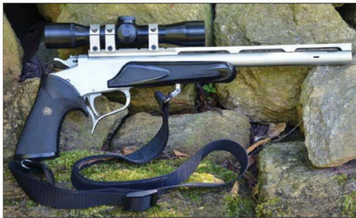
Layne's 14-inch SSK .375 JDJ barrel has a full-length rib with integral T'SOB scope mounting base. It is shown here with one of a limited run of Contender "flat-side" (no etching) frames, Pachmayr rubber grip and forearm, quick-detachable carrying sling and a Bausch & Lomb 2x handgun scope.
