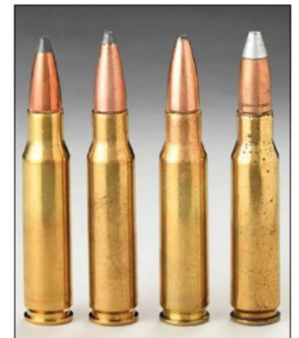
Some sources report that factory rounds can be measured for case expansion and then the handloader can use this measurement as a “do not exceed” level for load testing. These are the four factory rounds measured for case expansion.
