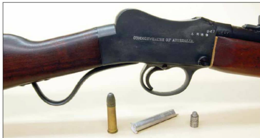
An Australian .310 Cadet “lightly sporterized” along with a factory cartridge, chamber cast and bore slug. All are mandatory if handloading is desired.
