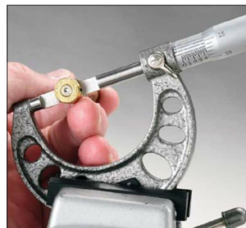
Even with the use of a vise, it is next to impossible to get repeatable measurements while properly positioning the case with one hand and keeping tension on the spindle ratchet with the other.
