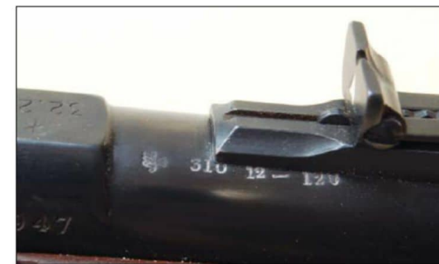
The factory cartridge marking on this Australian .310 barrel is partially covered by an added rear sight.
