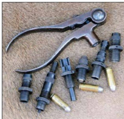
Instead of aluminum handles and four die sets as Mike used in the 1970s, this older 310 kit came with steel handles and a six die set.
