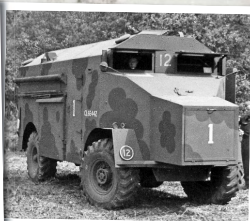
A version of the High Power Armoured Command Vehicle with an unusual nose on the front end.
