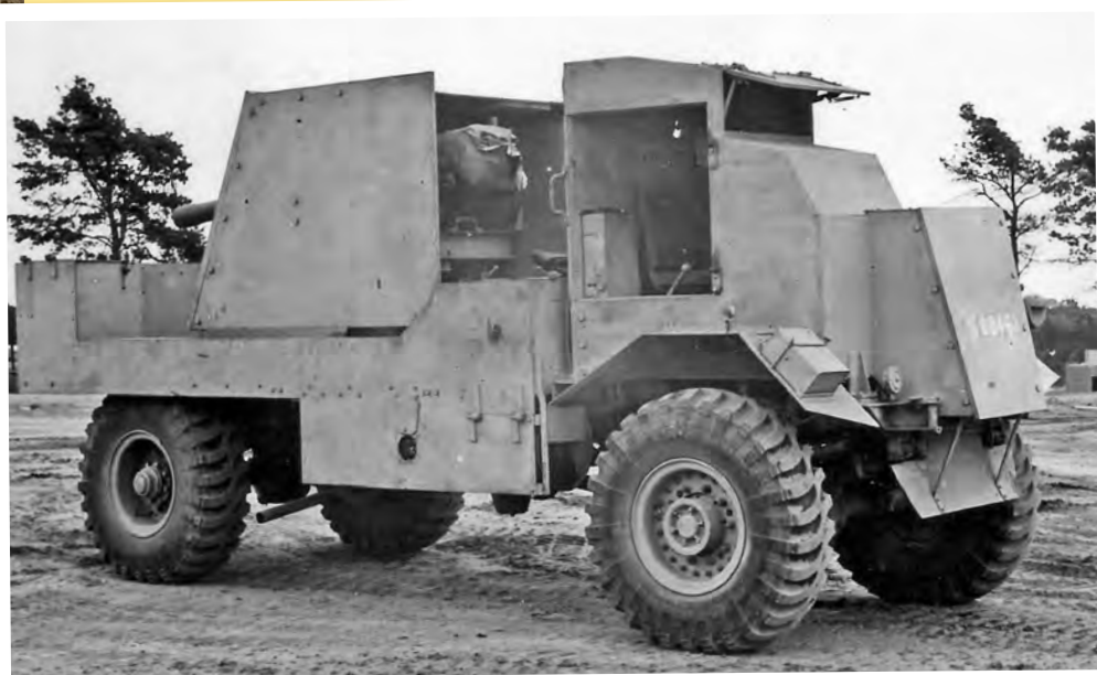
Right: The Armoured Mine Layer variant identified by the fact that someone has helpfully written ML at the front. This type was never developed.
