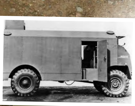
Above: The Armoured Demolition Vehicle version of the Dorchester showing the roof hatch through which a pile driver could be operated.
