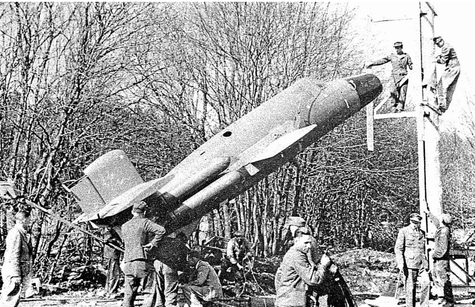
ABOVE: With Lothar Sieber dead, the Natter test programme reverted to unmanned testing. Here, vehicle M52 is winched into position on a newly designed single-rail tower.
