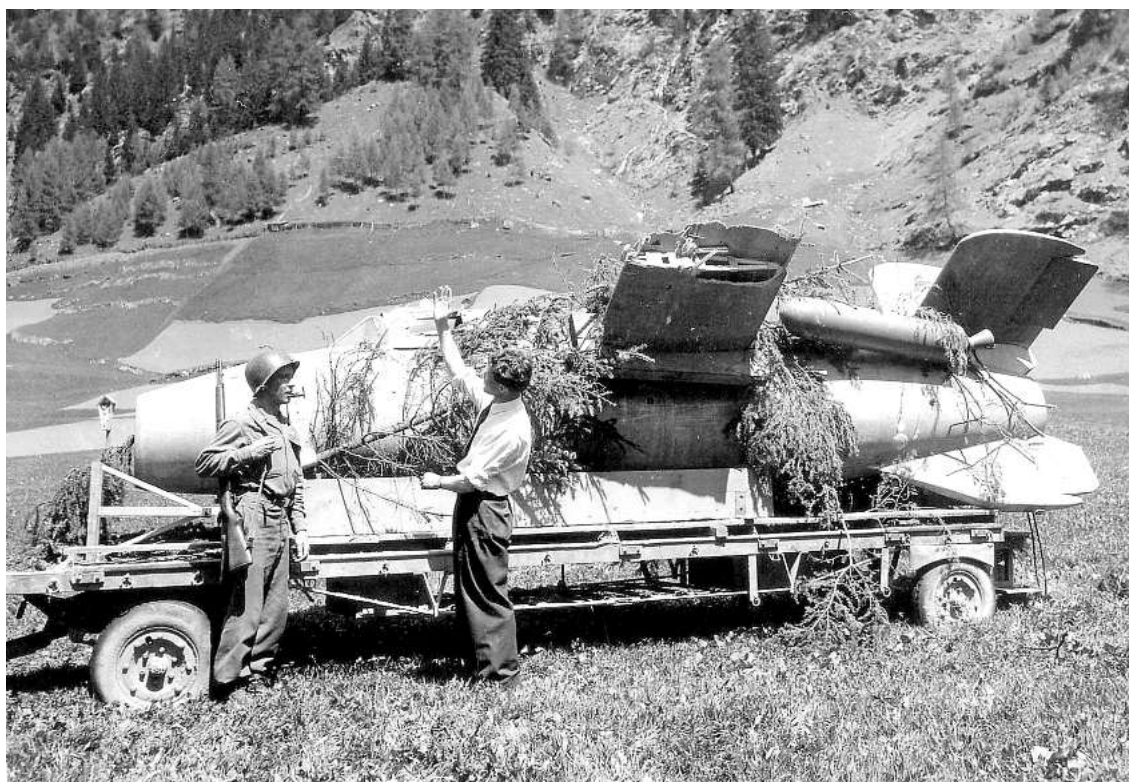
LEFT: Americans examine one of four damaged production Ba 349A-1 Natter aircraft captured in Austria.
