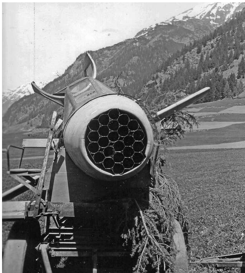
ABOVE: A frontal view of a Natter captured by the Americans, showing the honeycomb Föhn rocket launcher finally chosen as the aircraft's armament.
