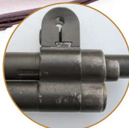
The muzzle of a "gas port" Garand (inset) will be familiar to most modern-day Garand owners. Ordnance Dept. drawings reveal internal views of the gas trap (below, L.) vs. gas port mechanisms.
