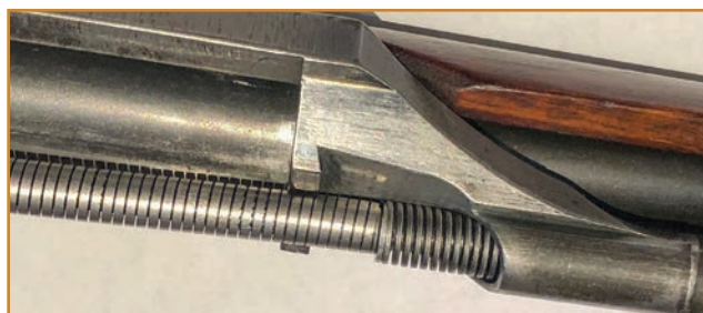
The follower rod on a gas trap M1 rifle is fitted with a "square wire" operating rod spring and separate compensating spring (above). Note how they differ from the follower rod and familiar "round wire" operating rod spring of a World War II-production M1 rifle, which is not accompanied by a compensating spring (below).
