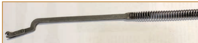
The follower rod on a gas trap M1 rifle is fitted with a "square wire" operating rod spring and separate compensating spring (above). Note how they differ from the follower rod and familiar "round wire" operating rod spring of a World War II-production M1 rifle, which is not accompanied by a compensating spring (below).
