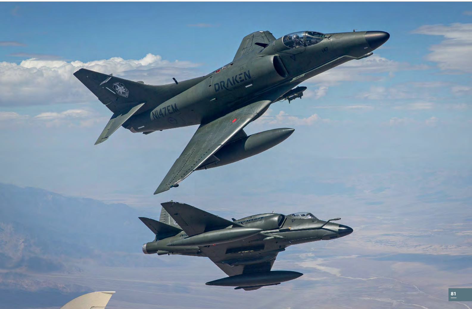
Top left: The Skyhawk nearest the camera is a former Israeli A-4N with extended jet pipe and a jammer pod under the centerline, with an ex-RNZAF A-4K leading the pair.
