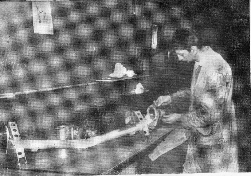
Eric Hind "miking-up" a ball-race housing on a de Dion tube from a DB3S.
