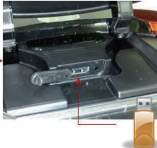
② Open USB cap and put USB memory that the program for black box upload is saved. Then close the cover
