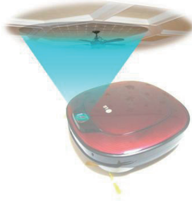
CV-SLAM Position detection and mapping A are performed at the same time from an image of ceiling
