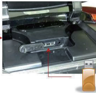
ⓑ Open USB cap and put USB memory that update program is saved. Then close the cover.
