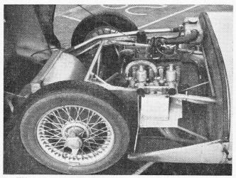
FULLY ACCESSIBLE, thanks to the completely detachable bodywork, the engine is revealed as that faithful work-horse, the Ford 10, with basic twin-carburetter modifications.
