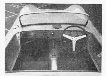
FUNCTIONAL cockpit layout contains all the necessary instruments and a small duralumin steering wheel with sponge-rubber rim, leather covered. The gear-change for the Ford box is of the Dellow type.
