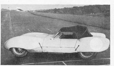
WEATHER protection includes a full width windscreen with wiper and a neat detachable hood with a large rear window. These pictures and the one opposite were taken at Brands Hatch.
